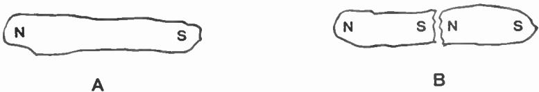
Figure 241. A—Poles on a magnet. B—Arrangement of poles on a magnet broken in half. Note that each piece has two poles.
