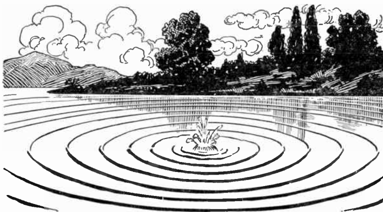
Figure 1. Ripples caused by throwing a stone into a still pond. These ripples travel in ever-widening circles from the point of disturbance.
