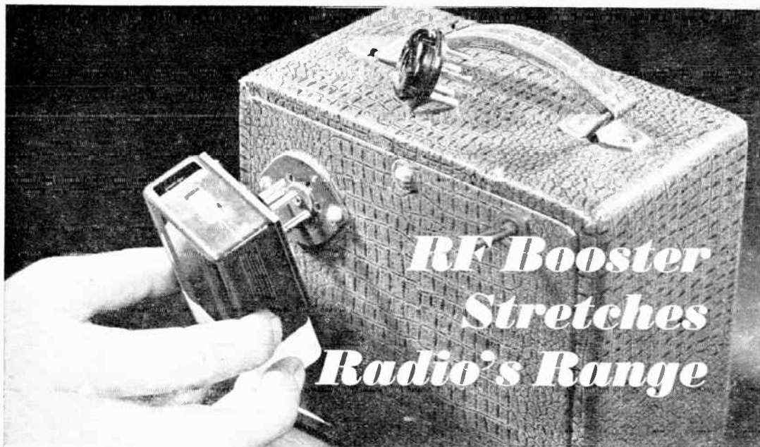
Plugging in an extra stage of amplification can improve the performance of small portables.
