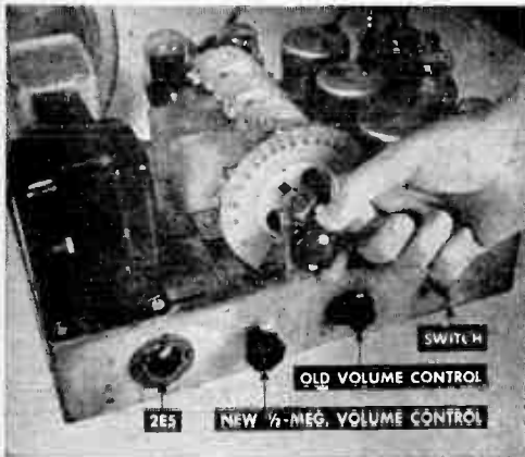
This 1931 model, 2-stage, TRF receiver first had to be altered for AVC and diode detection before a tuning eye could be made to operate.
