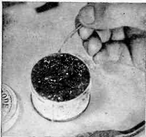
Copper wire solders best when it is tinned. Best bet is to buy it that way, but you can tin the ends yourself by scraping them clean
