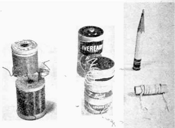
4. Coil forms can be improvised from many common objects. Windings must, of course, be figured in relation to diameter of the form. ▶
