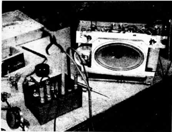
The pocket laboratory quickly tracked down the fault in this receiver. Used for stage-by-stage checking, it's a valuable service tool.
