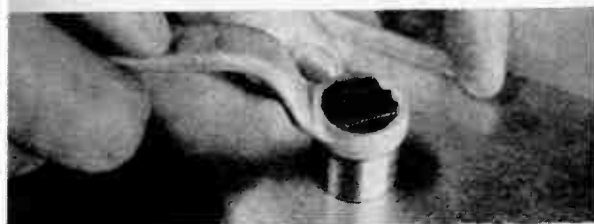
Drawing up the bolt with a wrench brings the cutter and die in contact with the chassis and shears out a clean, precise socket opening.
