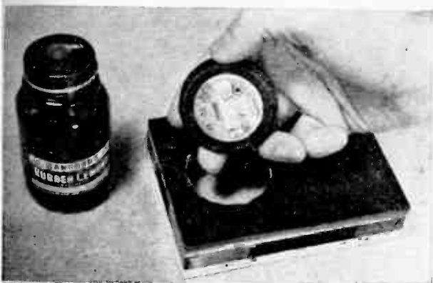
Cut a hole that will make a press fit for the rubber lip and cement the cartridge in place.
