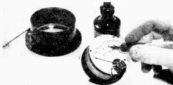
4. If a meter is altered to read 0.1 ma. by removing a shunt, the scale must be re-marked.
