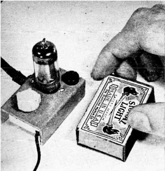
A shaft is soldered to the top of the trimmer condenser so that a tuning knob may be added.
