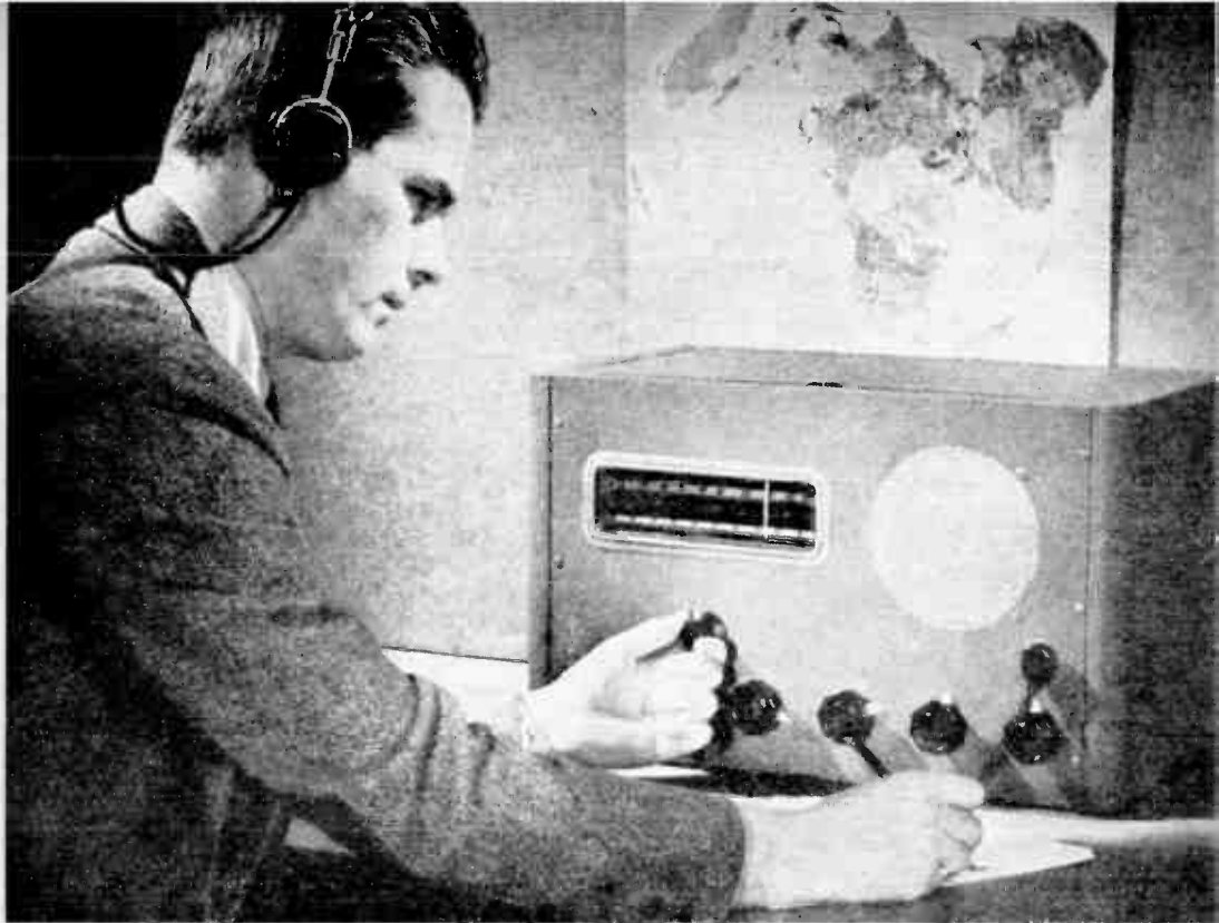
Elusive short-wave signals often come in best at night, so headphones are built into this two-band superheterodyne for midnight DX listening. Flicking a couple of switches, however, brings in the full broadcast band at loudspeaker volume.
