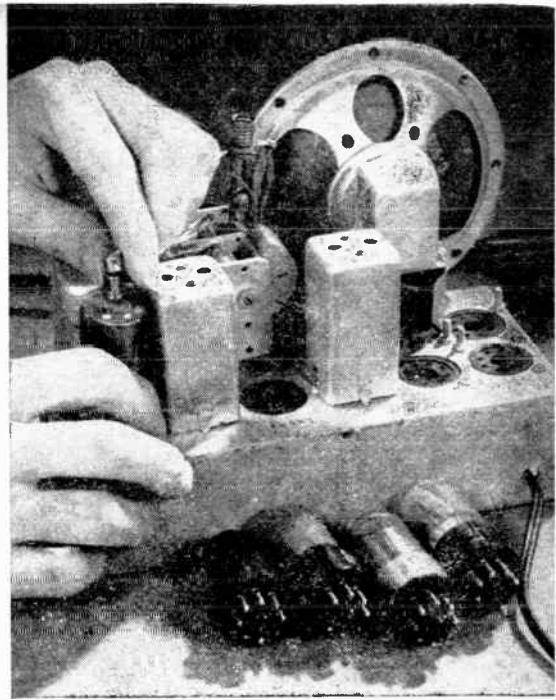
Tubes are fragile , so install them only after all the wiring is completed. The jumper lead from the RF section of C2 must be clipped to the grid cap of the 12A8 mixer tube.
