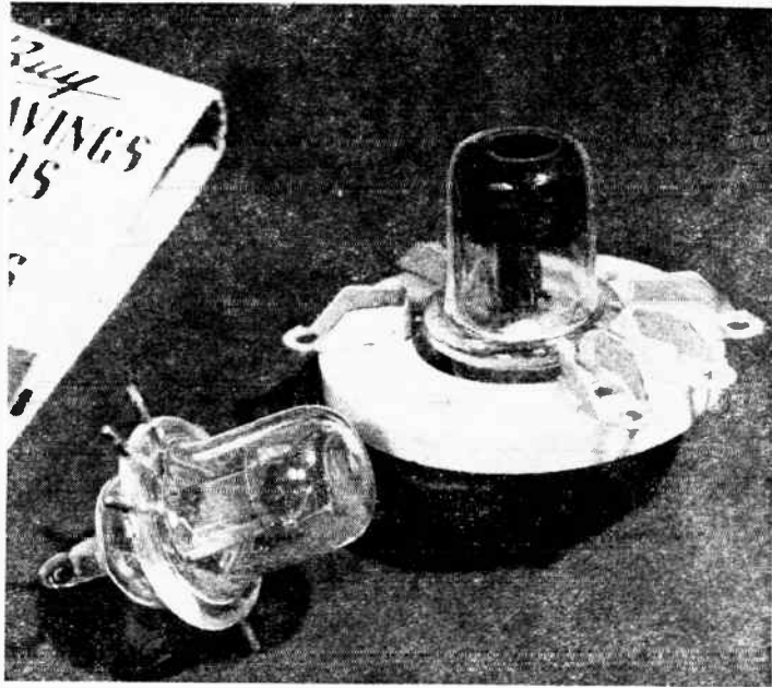
Shown full size, these tiny acorn triodes work at 500,000,000 cycles and more. In the socket is a 6-volt tube; the other is a 1 1/2-volt type.
