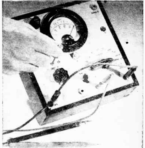
Adjusting the meter to read on the lowest ohm range. Scale divisions are graphed as below.
