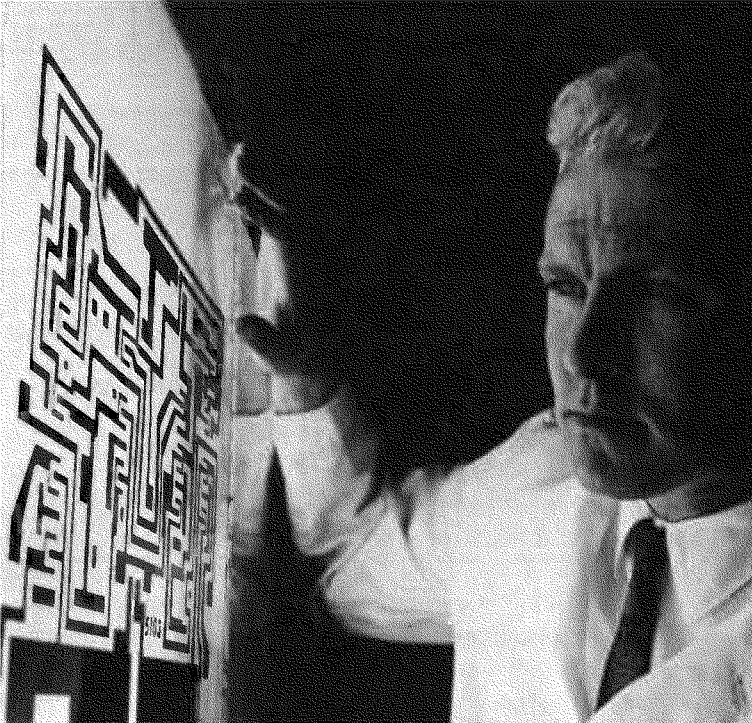
Fig. 1-5. A preliminary step in the manufacture of an IC is the large size pattern which will be reduced photographically on the silicon chip.
