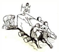
Put a pile of books on a table with a table-cloth, and it is difficult to slide them along. Put two or three round pencils under the bottom book and you can roll the pile of books easily. The lever and the roller are machines which make it easy to move things.
