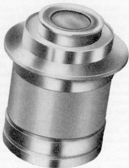
Fig. 16.1. Ceramic X-ray tube with a wide angle beryllium window for reproduction of Greuz Rays. Anode voltage 4 to 25 kv. Diameter of ceramic cylinder is 2 inch, over-all length 3\frac{13}{16} " 4 (Courtesy Machlett Laboratories, Inc.)
