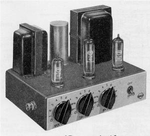
Prototype of Three watt Amplifier
