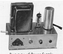
Prototype of Power Supply
