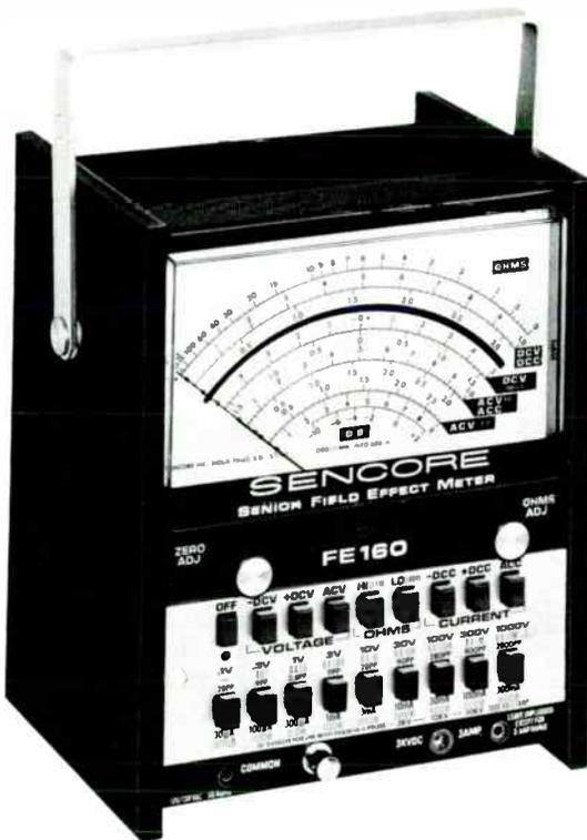
Fig. 2-16 A hi-lo FET multimeter. (Courtesy, Sencore)
