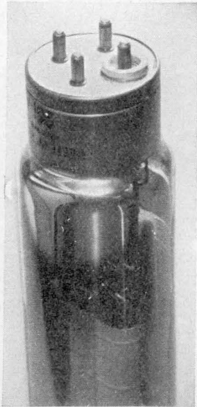
FIG. 7.—Barrier used to increase breakdown voltage across base of transmitting tube.
