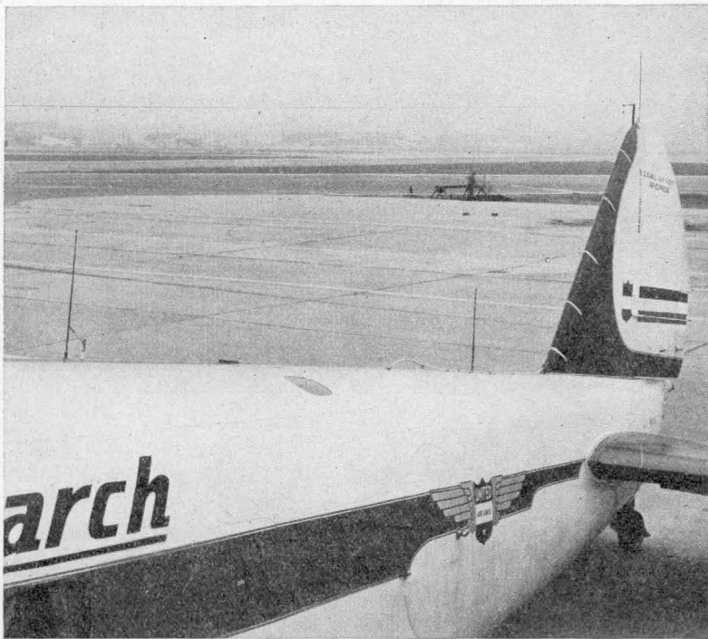
FIG. 183.—Various ultra-high-frequency communications antennas installed on airplane for tests. In the text the antenna immediately in front of the vertical fin is designated as No. 1, that behind the tail as No. 2, that located farthest forward as No. 3, and that mounted on the vertical fin as No. 4. (Courtesy United Air Lines.)
