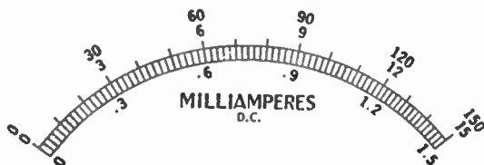
Fig. 6 Typical linear scale of multi-range DC milliammeter.
