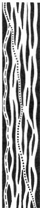
Fig. 32 Path of the playback stylus through the openings in the walls of a record which has been overcut.
