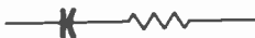
Fig. 1.—Representation of an imperfect capacitor as a perfect capacitor with series resistance.
