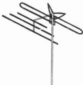
Fig. 89 Bat-wing antenna with reflector unit attached.
