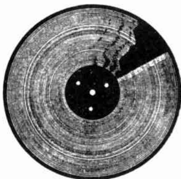
Fig. 35 A recording made on a defective blank illustrating the effect called "skip".
