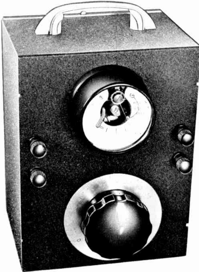
Figure 25. Front View of the Radio-Controlled Relay.
