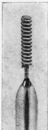
Fig. 73.—Electrode with Glass-like Coating for High-pressure Lamps (Osram, Berlin).
