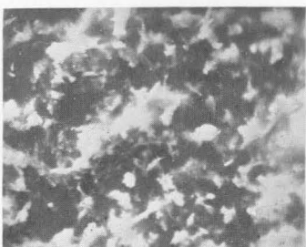
Fig. 18 (a) and (b).—Stereoscopical Microphotographs of Carbonate and Oxide Coatings before and after Decomposition (mag. \times 100 ).
