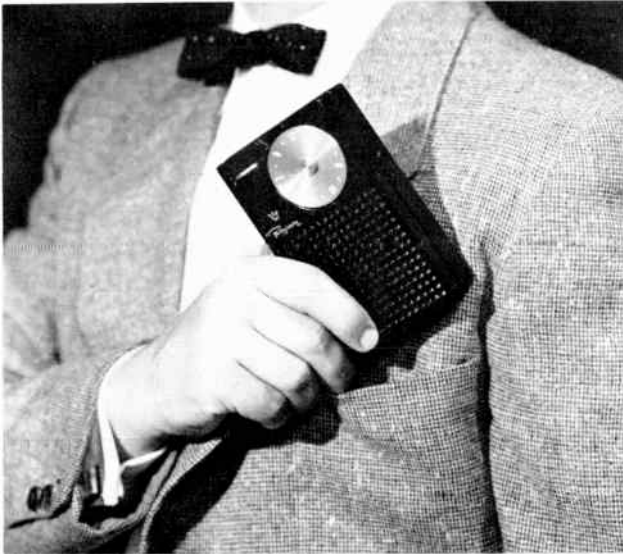
FIGURE 9.1 A transistor radio small enough to fit into the pocket of a man's jacket.
