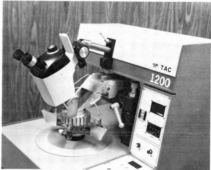
FIGURE 4.13 An automatic wafer prober. Automatic indexing with four-place accuracy is dialed into this wafer prober. Operator controls facilitates rapid orientation of wafer. (Courtesy Transistor Automation Corp.)
