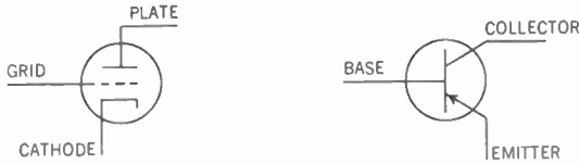
FIGURE 3.11 Comparable elements in tubes and transistors; grid and base, cathode and emitter, and plate and collector.
