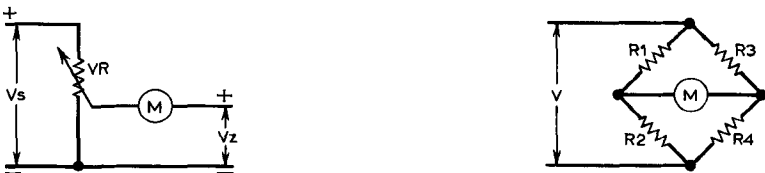
Fig. 1.5 (left) The Potentiometer. The variable resistor delivers a voltage V_s \cdot X , where X is the division ratio. If this equals V_z , the meter M is undeflected. The value of X can be read off the dial of the variable, and X \cdot V_s calculated.
