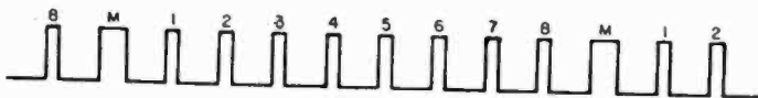
Fig. 8—Time-multiplex train of subcarrier pulses for 8 channels and marker pulse M for synchronization of receiver with transmitter.
