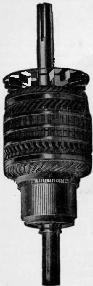
FIG. 366.—Western Electric barrel wound armature, having a fan attached at one end to induce a circulation of air for ventilation.
