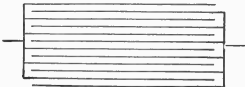
FIG. 141.—Conventional diagram of a condenser. A condenser is a device designed to absorb or hold an electric charge in about the same manner as a vessel will hold a liquid. Every conductor of electricity forms a condenser and its capacity for holding a charge depends upon the extent of its surface. A condenser is therefore made of conductive material formed into such shape as to present the maximum surface for a given amount of material.
