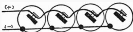
FIG. 73.—Diagram of a multiple or parallel connection. When connected in this manner the voltage of the battery is the same as that of a single cell, but the current is equal to the amperage of a single cell multiplied by the number of cells. Thus with 1\frac{1}{2} volt 15 ampere dry cells, the combination or battery connected as shown would give 4 \times 15 = 60 amperes at a pressure of 1\frac{1}{2} volts.
