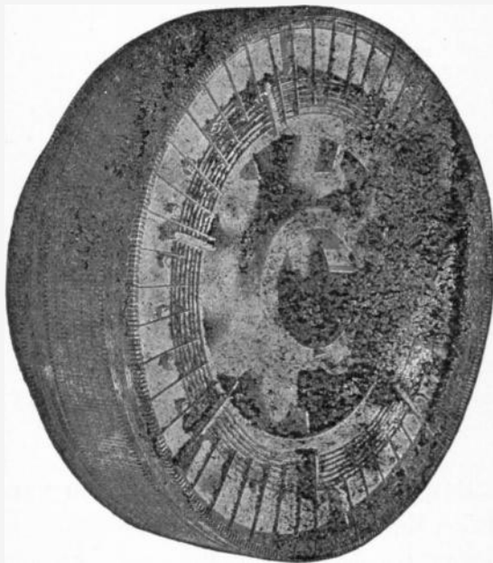
FIG. 278.—Rear view of armature of a large dynamo built by the General Electric Co., showing equalizer rings.
