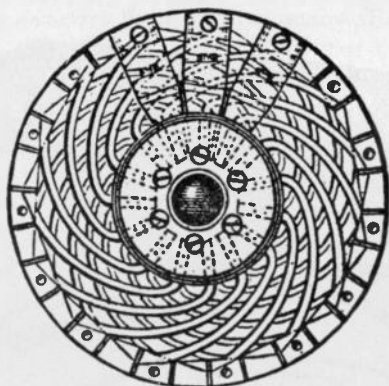
FIG. 374.—Siemens' bar armature; end view. Each inductor in the form of a bar is connected to the next by means of two evolute spiral copper strips, one bending inwardly, the other outwardly, their junction being in some cases secured to a block of wood upon the shaft. Their outer ends are attached to the bars by rivets or silver solder.
