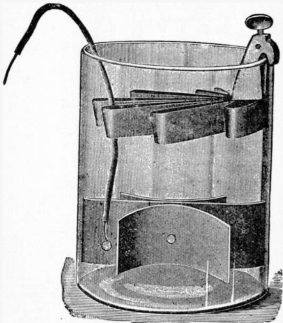
FIG. 53.—Daniell gravity cell, "crowfoot" pattern. This is a two fluid cell in which gravity instead of a porous cup is depended upon to keep the liquids separate. The two solutions consist of copper sulphate and dilute sulphuric acid, the elements being made of zinc and copper.
