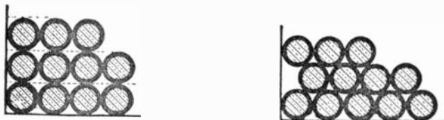
FIGS. 242 and 243.—Square and hexagonal order of "bedding." The term bedding is an expression used to indicate the relation between the cross sectional area of the winding when wound square, as in fig. 242, and where wound in some other way, as in fig. 243. In the square order of bedding, the degree of bedding equals zero.
