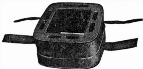
FIG. 246.—Fort Wayne compound wound rectangular ventilated spool field coil. The series and shunt coils are wound side by side, ventilating passages being provided lengthwise through each coil and between the shunt and series coils as shown.
