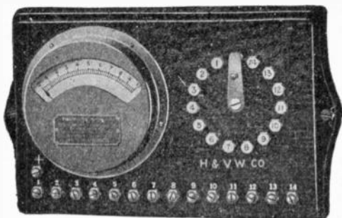
FIG. 4,556.—Waverly voltmeter with binding posts for fourteen tanks, thus enabling the operator to use only one instrument in obtaining the reading of any number of tank up to fourteen, by simply moving the switch lever to the tank numbers indicated on the switch of the instrument, and, when used in connection with tank rheostats, will enable the operator to reproduce at all times the same electrical conditions which by observation and experience he has found necessary in order to obtain a satisfactory deposit of uniform thickness and color in the shortest possible time.
