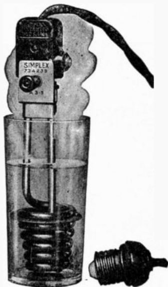
FIG. 4,411.—Simplex electric immersion heater. The most common way of boiling water is to apply heat to the outside of the vessel in which it is contained. But as heat radiates in all directions much of it is lost and only a part is usefully applied in heating the water. In other words when the heating agent surrounds the water only the heat that strikes in is used, that which strikes out is entirely lost. But if the water should surround the heating agent all the heat given off would be used. Advantage is taken of this fact in the Simplex heater by immersing the coil in a vessel of water.
