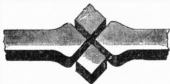
FIG. 4,483. Glut weld. A weld in which the ends of the two parts are tapered down, and the angles filled with wedges of iron, the whole being welded together while checking the length with a trammel, excess material being subsequently cut away. This type of weld is generally used in repair work where it is necessary to maintain unchanged the length of the broken part.
