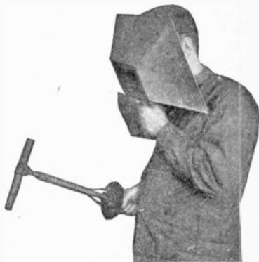
FIGS. 4,499 and 4,500.—C and C electric arc welding apparatus. Fig. 4,499, operator with one type of head shield and combination electrode holder for both metallic and graphite electrodes. Fig. 4,500, graphite electrode holder and hand shield.
