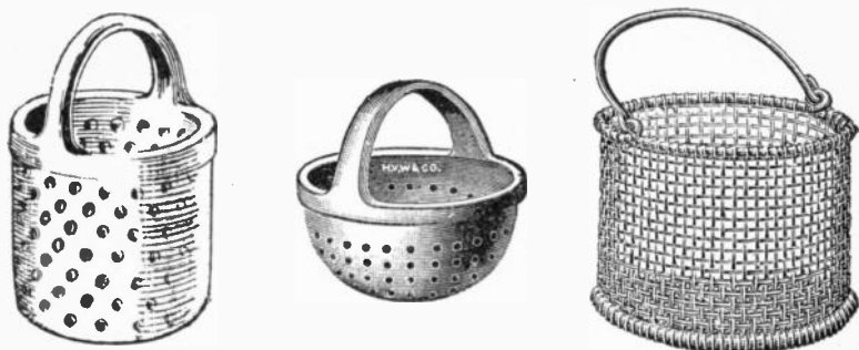
FIGS. 4,560 to 4,562.—Various dipping vessels. Fig. 4,560, deep glazed earthenware dipping basket; fig. 4,561, shallow glazed earthenware dipping basket; fig. 4,562, aluminum wire dipping basket. The aluminum basket is adapted for use in washing and dipping in all acid solutions, but cannot be used in potash solutions. Different shapes and sizes of basket are required for various kinds of work. Successful dipping depends, however, chiefly upon quick and careful handling rather than upon the shapes of the dip, therefore, the holes in these baskets should be as large as possible, so as to allow the acid or cyanide solution to drain out quickly.
