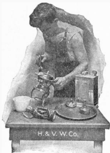
FIG. 4,575. —Method of applying lacquers. Instructions: Use a glass tumbler or porcelain cup as a container. Apply a flowing coat with a soft brush. A stiff brush will cause foaming or small air bubbles, and will require a heavier body lacquer. Prepare the work the same as for plating. It must be absolutely clean and free from grease or moisture. It requires only the smallest amount of moisture to ruin the work. Use the lacquer as thin as possible without showing iridescent colors. Dry in a temperature of 100° Fahr., if possible, using a thermometer. Brush lacquers will dry in the ordinary temperature, but baking improves the finish. Iridescent colors are in most cases caused by the lacquer being too thin, or by carelessness in removing the polishing composition or rouge from the work. Iridescent colors will often disappear when the article is given a second coating of lacquer after the first has dried. When the body becomes too heavy it needs thinner. Be sure to use only a thinner of the same grade as the lacquer.
