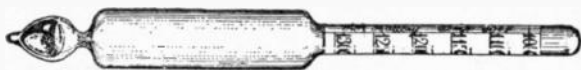
FIG. 4,623.—Acid hydrometer for testing the density of the electrolyte of acid electrolytic interrupters. It is important to have the specific gravity of the acid as follows: For a 110 volt current, 1,220; for a 220 volt current 1,070 Baume. The specific gravity can be approximately obtained by mixing ingredients according to the formula sent with the interrupter, but as this will vary from the evaporation of the water, it is advisable to use a hydrometer to determine when ( distilled ) water must be added, or when making a new solution. It should be noted that the reading of a hydrometer varies with the temperature, accordingly the reading must be corrected. Some hydrometers have a thermometer and correction scale in the neck.
