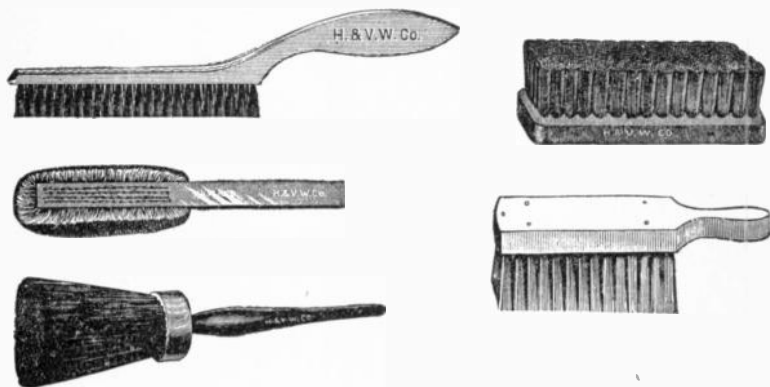
FIGS. 4,563 to 4,567—Various brushes. Fig. 4,563, jeweler's shoe handle wash out hand brush; fig. 4,564, flat scouring brush; fig. 4,565, cotton potash brush; fig. 4,566, sawdust brush; fig. 4,567, wire foundry brush.
