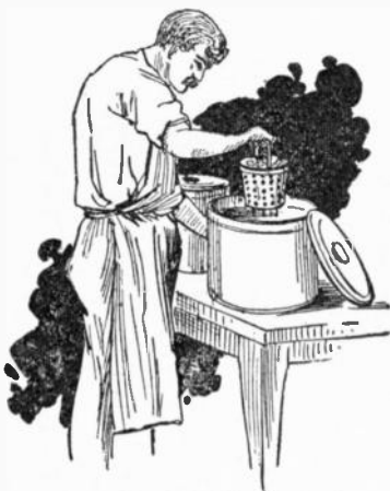
FIG. 4,595.—Dipping or immersion; a method of chemically cleaning many articles consisting of dipping them in solutions which dissolve the grease scale, etc. Successful dipping depends chiefly upon quick and careful handling rather than upon the dips themselves, and the holes in these baskets should be as large as possible to allow the rapid escape of acid or cyanide. The usual sizes of hole in dipping baskets are \frac{1}{8} , \frac{1}{4} , \frac{3}{8} , \frac{1}{2} , \frac{5}{8} , \frac{3}{4} , \frac{7}{8} , to 1 inch in diameter.
