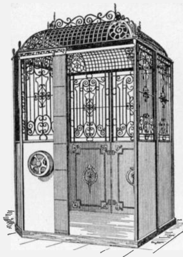
FIG. 4,128.—Typical modern passenger car. Wood or other combustible material is practically eliminated, and with the exception of the floor boards, the construction is all metal. Sheet metal is employed around the lower part and open metal grill work around the upper portion giving a well ventilated and light yet strong car.
