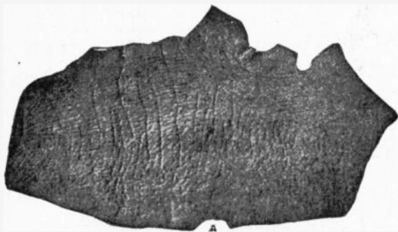
FIG. 4,594.—Walrus or sea horse leather. Walrus leather has a peculiarly tough grain making it especially adapted for polishing wheels. It is extensively used for polishing iron, steel, brass, cutlery, silverware, etc., where a fine polish is required. It can be used with emery, crocus, rouge, or rotten stone and gives a smooth fine finish to the work. The leather is used in the form of solid wheels or cut into strips which are used for covering wood wheels. Walrus hides are invariably uneven in thickness and in order to avoid any misunderstanding as to thickness when purchasing, it has long been a recognized custom of the trade to measure the thickness at the part of the hide marked A.
