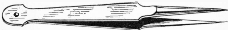
FIG. 4,471.—Brazing the joint of a pair of tweezers. The surfaces to be brazed are cleaned, some of the spelter applied to each surface, and the pieces tied together with a fine iron wire and heated sufficiently to melt the spelter. The heat may be applied with a blow pipe or by holding the pieces in a pair of hot tongs. When the spelter is melted the piece is cooled and the iron wire is taken off. When the pieces are clamped in hot tongs, the tongs depended on to keep them there, or stops may be arranged to determine the location of the pieces.
