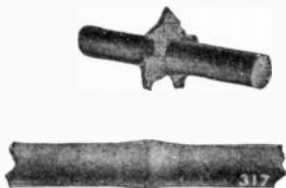
FIGS. 4,517 and 4,518.—Flash weld, and upset weld. A flash weld is generally used on stock that is wide and thin; where it is rectangular in shape, and where it is not possible to have the welding faces cut square and true. Also in welding tubing to forgings, or tubing to tubing. In all cases where a small amount of stock is to be taken up in welds, or when it is desired to shear or grind off the fin, a flash weld is made. Upset welding is used in all cases where the weld is to be hammered, using the heat generated in the welding. Also for small rods or rings where it is not necessary to have a uniform thickness of stock. On brass or copper a flash weld is made. Three times the diameter of stock between the dies should be allowed on brass and four times on copper, but only once the diameter of stock is actually taken up in the weld.
