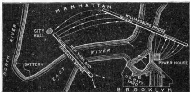
FIG. 4,530.—Electrolysis in lower New York. The figure illustrates current movements as discovered. The power house is located near the navy yard in Brooklyn. A portion of the returning currents, as shown by arrows, flows over the New York and Brooklyn bridge to Manhattan, thence north to Williamsburg bridge via underground mains, subway structures, and other metals, and passes over that bridge back to Brooklyn, thence through mains to rails and negatives, to power house. In this case damage may be expected at three points: 1, where currents leave bridge metals on the Manhattan side; 2, where they leave pipes to enter Williamsburg bridge; 3, where they leave same bridge for pipes in Brooklyn side. When the two bridge structures are connected in Manhattan as proposed, then there will be further changes in the direction of current. Before the Williamsburg bridge was built, these currents recrossed through the river bed, leaving mains all along the docks in the Manhattan side, for the river, and leaving the river for mains or other metals along the docks of the Brooklyn side. Traces of these currents have been found as far north as 23d st., a distance of over two miles from the Brooklyn bridge. Since the Williamsburg bridge has been built, nearly all traces of these currents flowing north of it have disappeared, showing that the mass of metal composing the structure acts as a short circuit or path of lower resistance which carries practically all of the returning currents flowing from Manhattan back to Brooklyn.
