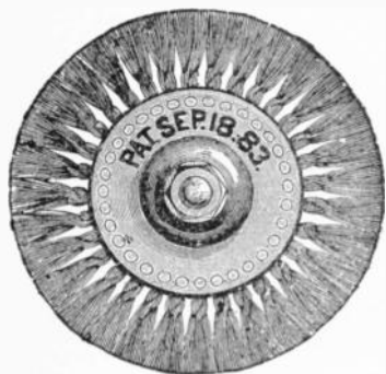
FIGS. 4,568 to 4,571.—Hanson and Van Winkle swing type, circular steel wire, casting brush. The steel wires are twisted in knots and the knots are hung on rods around the hub, as shown in fig. 4,571, so that they will turn around the rods if the work be held too close to the brush wheel. In using the brush the work should be held so as to be just in contact with the ends of the wires. The brush shown is about 15 inches in diameter, and should not be run much faster than at the rate of 1,000 revolutions per minute. If the brush be run too fast, or if the work be held too close, the wires will become crystallized and soon break off. After the brush has been run for a while, the ends of the wires will become bent and drag over the surface of the work; the brush should then be taken off the spindle, turned around, and replaced with the hub next to the collar on the spindle, so that the wire ends will again strike the surface of the work. When the wires are worn out a new set of knot can be readily substituted for the old set by unscrewing the nut N and taking off the hub plate P.
