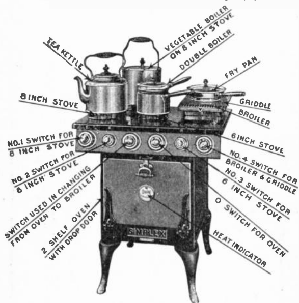
FIG. 4.414.—Simplex electric range consisting of oven, broiler, toaster, and two or more disc heaters with separate cooking utensils. Heating in top and bottom of oven are controlled by a three heat switch. The broiler has a corrugated top slanting slightly toward a grooved end which receives the juices of the meats. A separate smooth top fits on the broiler for making griddle cakes, toast, etc.
