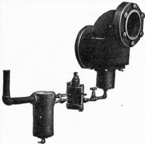
FIG. 4,381.—Ingersoll-Rand Imperial unloader. It operates by closing the air intake, and automatically regulates the compressor, maintaining the line pressure within a satisfactory range. It consists of a valve on the compressor intake pipe, normally held open by its own weight. When receiver pressure rises above normal this pressure is communicated through a small pipe from the regulating valve, acting to close the valve in the intake pipe, thus shutting off the air supply. The regulating valve can be adjusted for any working pressure by means of a spring adjusting screw.
