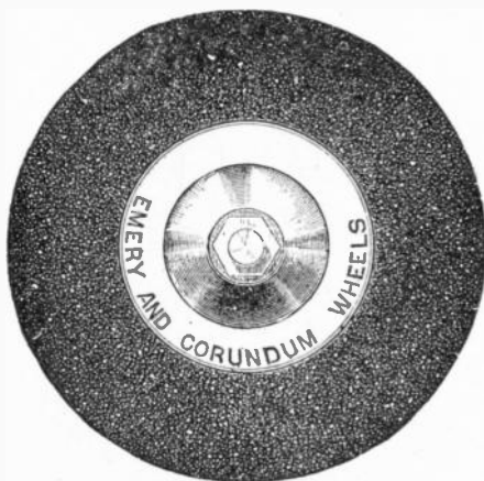
FIG. 4,579.—Emery and corundum wheel. Grade 1 is soft and suitable for grinding planer knives, paper cutting, and leather splitting knives, light surface work and roll grinding. Nos. 36 to 60. Grade 2 is for gumming saws, and rough chilled roll grinding. Nos. 36 to 60. Grade 2½ is for grinding moulding cutters, and wood working tools generally, soft steel, mouldboards of plows, and surface work on brass and iron. Nos. 20 to 60. Grade 3 is medium and suitable for grinding machine shop tools, tool steel, twist drills, surface work, polishing the edges of stoves, and will do a greater variety of work than any other grade. Nos. 30 to 70. Grade 3¼ is somewhat harder than grade 3, and is used for tool grinding in machine shops. Nos. 36 to 60. Grade 3½ is for rough work in a machine shop, brass castings, malleable iron, soft foundry castings, ivory, horn, and shell grinding. This is a fast cutting wheel. Nos. 36 to 60. Grade 3¾ is used for general grinding in foundries; is a faster cutting wheel than grade 4 and is more in use. Nos. 16 to 24. Grade 4 is medium hard and is adapted to grinding heavy iron castings, malleable and wrought iron, steel castings, stove work, and sprues and gates from heavy castings. Nos. 16 to 24. Grade 4¼ is a hard wheel, to be used on heavy iron and steel castings, when a faster cutting wheel than grade 4½ is required. Nos. 16 to 20. Grade 4½ is hard and adapted to grinding heavy iron castings and edge work on iron and steel. Nos. 16 to 20. Grade 5 is very hard. This wheel is made especially for plow jointing and very hard steel edge grinding; will not do surface work. Nos. 16 to 20. Grade 6 is made of the finer grades of emery, to be used where there is not much metal to be removed, and where the wheel is expected to retain a certain shape, as in grinding flutes of taps, milling cutters, etc. Nos. 60 to 120.
