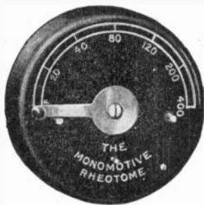
FIG. 4,628.—McIntosh monomotive rheotome, for interrupting galvanic, faradic, or sinusoidal current for therapeutic application. The range of interruption is from 20 to 400. The instrument consists of a clock work mechanism with platinum tipped contact, and is wound up with a key, running 45 minutes with a single winding. In adjusting , a lever is turned to the frequency desired; this movement of the lever turns on the clock mechanism, selects the frequency and places the rheotome in the circuit. Turning the lever back to the "off" point similarly cuts it out of circuit and stops the mechanism. The motion of the spring is impeded by a fan, hence the resistance is the same in either horizontal or vertical position. In connecting , it is placed in series between the patient and battery or other apparatus.
