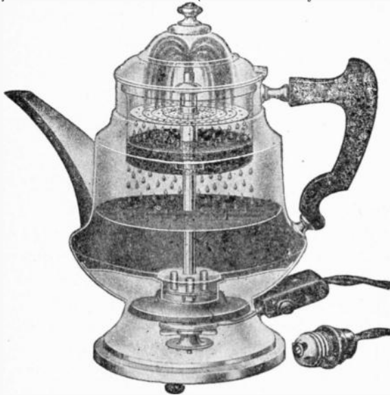
FIG. 4,388.—Simplex electric coffee percolator. Starting with cold water, through the circulating process as shown, drip coffee is ready in a few minutes, depending upon the degree of strength required. Three degrees of heat are provided, permitting quick making, and allowing the coffee to be kept hot at the lowest current consumption.
