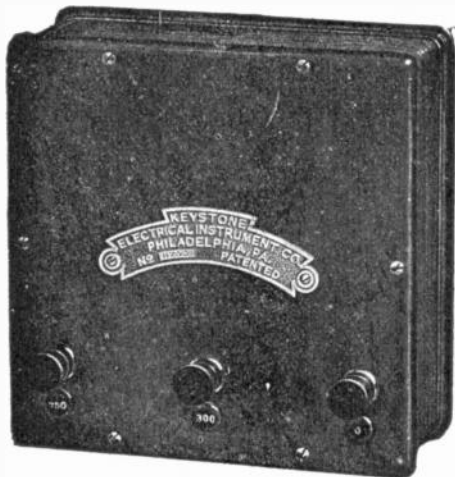
FIG. 643.—Portable multiplier for portable voltmeter. A multiplier is used for increasing the readings of voltmeters, and consists of resistance coils placed in a portable case. A multiplier is connected in series with the voltmeter and must be adjusted for the instrument with which it is to be used, because the resistance coil must be a multiple of the voltmeter resistance. For instance, a multiplier with a value of 10, used with a 6 volt voltmeter or 521 ohms would measure about 5,215 ohms; one with a value of 40, would equal about 20,860 ohms. The multiplier 10 would give a total scale value of 60, and the multiplier 40, a total scale value of 240 volts to the 6 volt instrument. A multiplier is of considerable value in that it does away with the necessity of having a number of voltmeters of different ranges. The instrument here illustrated has a range of 150 volts.
