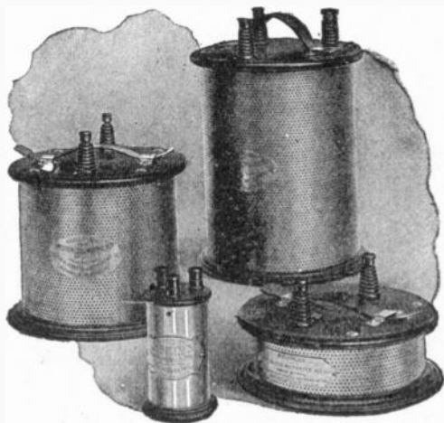
FIG. 641 to 642.—Multipliers for Weston standard portable voltmeters. Multipliers are resistance boxes, the coils in which are highly insulated, and are adjusted so that the readings of the instrument may be multiplied by any desired constant. Multipliers are usually constructed so that the indications of the pointer, multiplied by 2, 5, 10, 20, or 50, will give the voltage of the circuit. By the use of multipliers the range of voltmeters may be increased to any practical limit.
