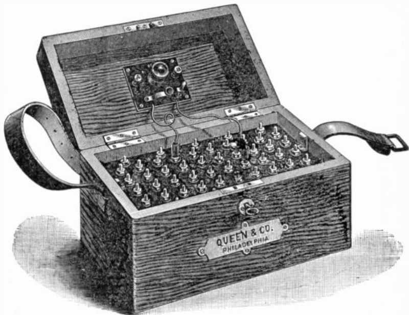
FIG. 580.—Queen portable silver chloride testing battery. The silver chloride cell has the advantage of long life, light weight, and compactness. The pressure of each cell when new is .8 volt.
