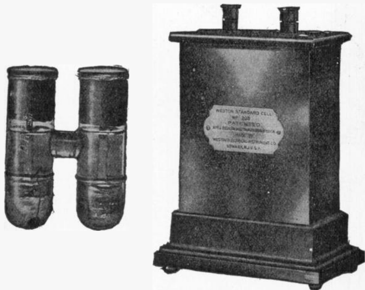
FIG. 541. —Weston Cadmium Cell. It is made in two forms; one known as the Weston normal cell, in which the solution of cadmium sulphate is saturated at all temperatures at which the cell may be used. The other, known as the Weston standard cell, in which the cadmium sulphate solution is unsaturated at all temperatures above 4^{\circ}\text{C} . The Weston normal cell, or saturated form is slightly affected by changes in temperature, but, on account of the fact that it can be accurately reproduced, it was adopted by the London Conference in 1908, as a convenient voltage standard. The value of its voltage suggested by the committee of the London Conference on Electrical Units and Standards, and adopted by the Bureau of Standards at Washington, Jan. 1st, 1911, is 1.0183 International volts at 20^{\circ}\text{C} . At any other temperature its voltage is:
