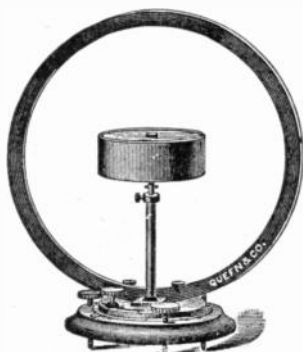
FIG. 522. —Queen tangent and sine galvanometer. This instrument properly adjusted can be used as a standard instrument for laboratory work. The brass ring is 12 inches in diameter, and the grooves in which the wire is wound are carefully turned so as to be of true rectangular cross section, thus allowing the constant of the instrument to be accurately calculated and compared with the constant as obtained by other methods. The compass box is 5 inches in diameter and is so held in position that it may be raised or lowered, rotated on its vertical axis, shifted out of the plane of the coil, etc., thus enabling the operator to acquire proficiency with the instrument and to meet all cases of derangement possible. The dial is graduated to single degrees, and the needle is suspended by a very light cocoon fibre. The whole instrument can be turned about its vertical axis, and a quadrant graduated in degrees upon the base allows the amount of rotation to be accurately measured, and the laws of the sine galvanometer investigated. The instrument is wound to measure .25 ampere to 8 amperes.
