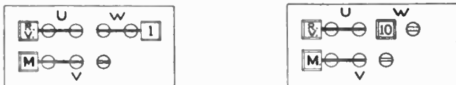
FIG. 605.—To use galvanometer of Leeds and Northrup fault finder in series with the battery: Set switches as shown, and connect between posts Gr. and 2 (see figs. 587 and 588). The galvanometer will have the maximum sensibility with the pointer at 1,000 and the minimum at zero.
