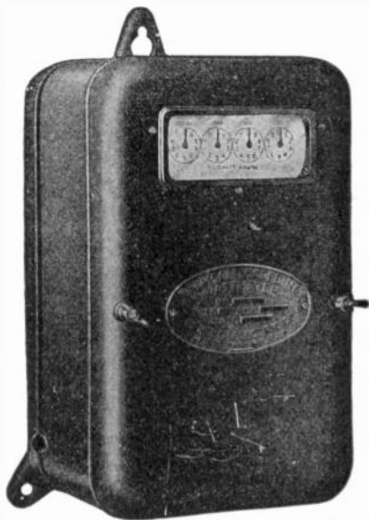
FIG. 653.—Thompson watt hour meter (type C-6). This form is furnished with side connections, the line wires entering at the left and the load wires at the right. Both sides of the system are carried through the meter in all sizes up to and including the 50 ampere size. In meters of larger ampere capacities, a voltage tap is used.
