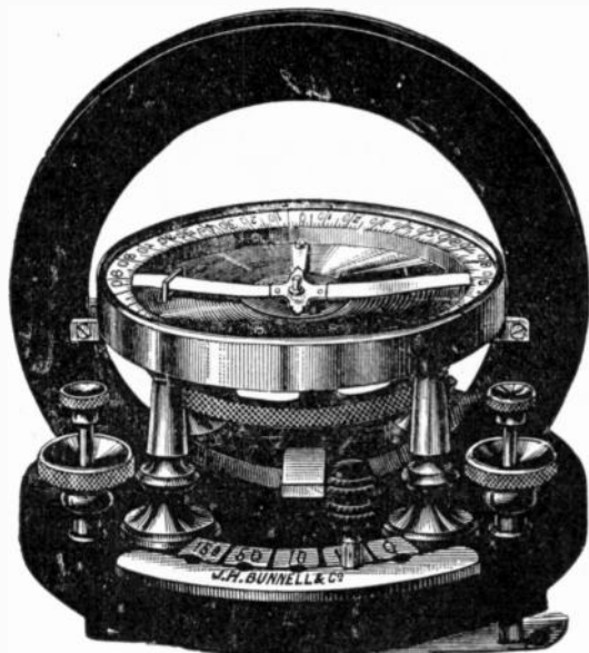
FIG. 515. —Bunnell tangent galvanometer. This instrument is mounted on a circular hard rubber base, 7\frac{1}{4} inches diameter, provided with levelling screws and anchoring points. The galvanometer consists of a magnetized needle \frac{1}{8} inch in length, suspended at the center of a rubber ring six inches in diameter, containing the coils. There are five coils of 0, 1, 10, 50 and 150 ohms resistance. The first is a stout copper band of inappreciable resistance; the others are of different sized copper wires, carefully insulated. Five terminals are provided, marked, respectively, 0, 1, 10, 50 and 150. The ends of the coils are so arranged that the plug inserted at the terminal marked 50 puts in circuit all the coils; marked at the terminal 50—all except the 150 ohm coil; and so on, till at the zero terminal only the copper band is in circuit. Fixed to the needle, which is balanced on jewel and point, is an aluminum pointer at right angles, extending across a five inch dial immediately beneath. One side of the dial is divided into degrees; on the other side, the graduations correspond to the tangent of the angles of deflection.
