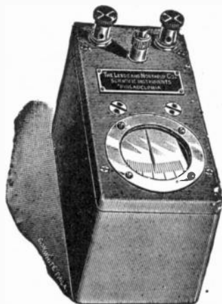
FIG. 559.—Leeds and Northrup portable galvanometer (pointer type A). The sensitiveness of this instrument is such that it may be substituted in numerous cases for the non-portable reflecting type of galvanometer; as for instance, in the checking of ammeters and voltmeters to an accuracy of .2% by the potentiometer method, and on almost all Wheatstone bridge measurements to commercial accuracies. A current of 2 micro-amperes will cause the pointer to move 1 mm. over the scale, that is, it has a sensibility of 500,000 ohms. The method of suspending the moving system is such as to practically eliminate initial friction which is of value in all zero deflecting methods. The suspensions and moving system are guarded by springs, which together with the solid construction of the case, render the instrument capable of withstanding rough usage. Overall dimensions are 5\frac{1}{4}'' \times 2\frac{3}{4}'' \times 3\frac{1}{2}'' ; weight about 3 pounds.
