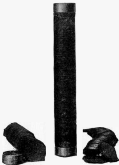
FIG. 747.—Allen-Bradley compression type resistance units. The contact resistance between the discs composing the resistance column is subject to variations of pressure, thereby producing proportionate resistance changes in the column as a whole. In the complete resistance unit, the resistance column is encased in a drawn steel tube, which is lined with a highly refractory cement, for purpose of insulation, affording the column both mechanical and electrical protection and excluding the air which effectually prevents any combustion should the column become red hot due to overload. The ends of the tube are closed by means of caps through which pass electrodes for making connections between the discs and exterior conductors. The steel tube, when necessary, is provided with ribs or fins for the dissipation of acquired heat.
