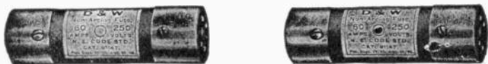
FIGS. 479 and 480.—D & W fuse indicator. The operation is illustrated in the figures which show appearance of the label before the blowing of the fuse, fig. 479, and the same fuse blown, as indicated by the appearance of the black spot within the circle fig. 480.
