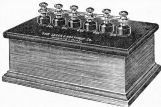
FIG. 561.—Megohm box or set of standard high resistances. The box contains five resistances of 200,000 ohms each. The six pillars are petticoat insulated, the resistances being placed between each pair of pillars. There is a double contact post on top of each pillar so that these can be connected together with copper links.
