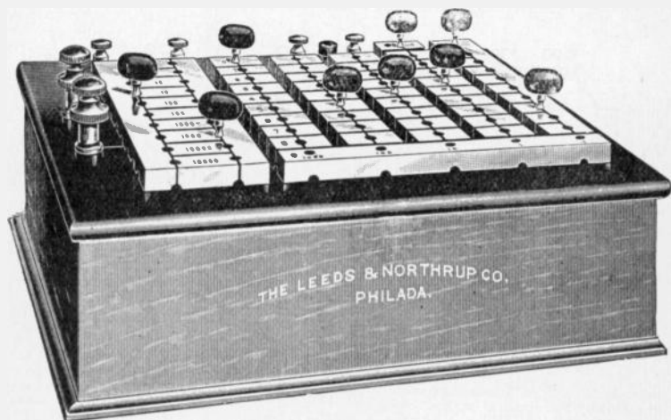
FIG. 567.—Standard resistance box and Wheatstone bridge. This pattern is a modification of the Anthony form of bridge. All the resistances are wound upon metal spools. The bridge ratio coils are 1, 10, 100, 1,000, 10,000. The rheostat coils are arranged in five rows, of ten coils each. The ordinary decade plan (explained in fig. 570) is followed. The coils may be joined in series in multiple, or in any combination of series and multiple. The coils may thus be checked against each other in many combinations. For instance, all the ten ohm coils taken in parallel may be compared with any one ohm coil. The precision of adjustment is said to be \frac{1}{20}\% for the coils of the tenth ohm series, and \frac{1}{50}\% for the coils of the rheostat. The ratio coils are certified to be like each other to within \frac{1}{100}\% . The box is supplied with battery and galvanometer keys of substantial construction.
