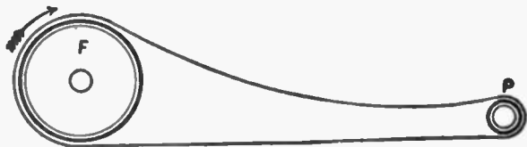
FIG. 448.—Right way to run a belt. The pull should come on the lower side bringing the slack on top.
