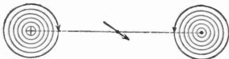
FIG. 517.—Horizontal section through middle of tangent galvanometer, showing magnetic whirls around the coil and corresponding deflection of needle.
