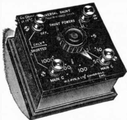
FIG. 539.—Ayrton-Mather universal shunt. This shunt may be used with any galvanometer. The total resistance is 10,000 ohms, with shunt powers of 1, 5, 10, 50, 100, 500, and 1,000. It is also fitted with positions in which the galvanometer is shorted and off. The coils are of constantan wire.
