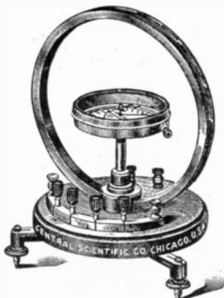
FIG. 514.—Central Scientific Co. tangent galvanometer. A 9 inch brass ring is mounted on a mahogany base which rotates on a tripod provided with levelling screws. The needle has an aluminum pointer and jewelled bearing. The winding consists of 300 turns of magnet wire so connected to the plugs in front that 20, 40, 80, or 160 turns or any combination of these numbers may be used. For heavy currents a band of copper is used by connecting to the extra pair of binding posts in the rear of the instrument.
