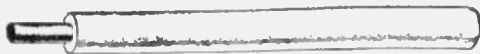
FIG. 810.—Slow burning wire, formerly known as Underwriter's Wire. The insulation is triple braided, saturated with a white fireproof compound. Solid conductor.
