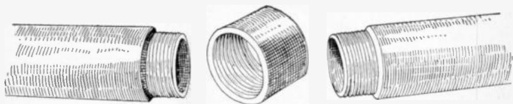
FIG. 986.—Screw joint type of fibre conduit. This method of connection will form a tight joint and is suitable for running under the lawns of private houses and parks, under the streets of towns and villages, and in other places where the cost of building electric subways is prohibitive.
