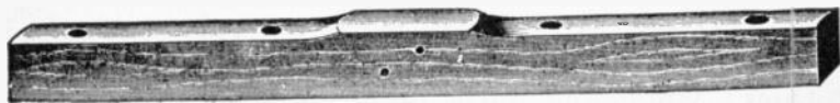
FIG. 936.—Cross arm which carries the insulator pins. The standard cross arm is 3\frac{1}{4} x 4\frac{1}{4} inches, double painted, and bored for 1\frac{1}{2} inch pins and two \frac{1}{2} inch bolt holes. Telephone arms are 2\frac{3}{4} x 3\frac{3}{4} inch, bored for 1\frac{1}{4} inch pins and two \frac{1}{2} inch bolts.
