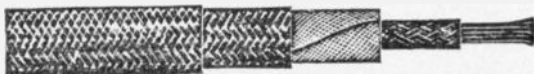
FIG. 813.—Gas engine ignition cable. This is a special cable made to stand the hard service necessary on automobiles. The conductor is composed of 36 strands of No. 27 tinned copper wire, equal to No. 14 in capacity, which gives it necessary flexibility. About this conductor are woven two layers of cotton thread. Over this are woven, in opposite directions, several layers of specially prepared tape which has been given two coatings of fine insulating varnish. Two strong braids of cotton form the outside covering, and each of these different braids is passed through a bath of insulating liquid and baked in a steam heated oven. With three layers of tape the cable will stand a test of 18,000 to 20,000 volts, and with five layers, 30,000 volts.
