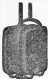
FIGS. 1,086 to 1,089.—The "Champion" Accumulator; views showing parts and assembly. Fig. 1,086, empty plate; fig. 1,087, filled plate; fig. 1,088, complete element, small type; fig. 1,089, cell assembled. The plates are of the envelope type and are made thick. The active material is held firmly in place by a covering of lead. A few thick plates are used instead of many thin ones.
