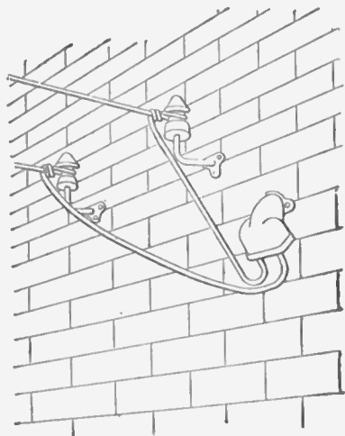
FIG. 903.—Service entrance to interior conduit system; showing method of preventing moisture reaching the interior of the conduit system.
