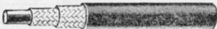
FIG. 811.—Slow burning weather proof wire. The insulation is composed of two braids thoroughly saturated with a fire proof composition, over which is a highly polished weather proof third braid. This wire was formerly known as "fire and weather proof" wire.
