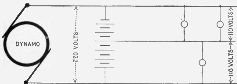
FIG. 1,183.—Diagram showing three wire system with one dynamo and storage battery. A 220 volt dynamo charges a storage battery of corresponding pressure, which in turn subdivides the pressure and supplies a three wire system, the neutral wire of which is connected to the middle point of the battery as shown.
