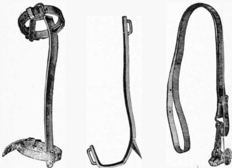
FIGS. 950 to 952.—Lineman's tools. Figs. 950 and 951, Eastern pole climbers, with and without strap for attaching to legs; fig. 952, portable vise with strap for pulling up the slack in splicing.
