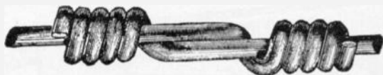
FIG. 961.—American wire joint. This is a simple method of connecting the ends of the sections of wire by tightly twisting the ends around each other for a few turns; it is the standard Western Union wire joint.
