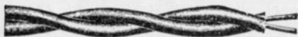
FIG. 815. —Pothead wires. The standard wire for pothead work is either No. 19, 20 or 22 B. & S. gauge, either single conductor or twisted pair, insulated to a diameter of \frac{1}{2} inch over rubber, without any outer braid or protection. In the case of twisted pairs one conductor is usually made of a differently colored rubber than the other, so as to distinguish between them.
