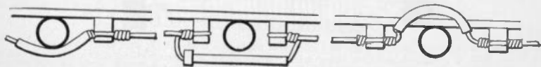
FIGS. 851 to 853.—Methods of wiring across pipes. The wires should preferably run over rather than under the pipes. Fig. 851 shows crossing with circular loom, and fig. 852, one in which a tube is used. Both of these methods are satisfactory in the case of gas pipes, but for steam pipes or water pipes which are liable to leak or sweat and drip moisture, the crossing should be above as shown in fig. 853. On side walls where vertical wires run across horizontal water pipes, the latter should be enclosed and the moisture deflected to one side.
