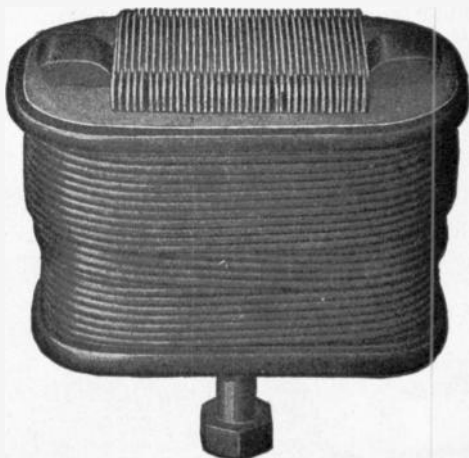
FIG. 1467.—General Electric field coil, showing one method of winding. In the smaller machines the wire is wound on spools which are slipped over the pole pieces, which are built of sheet iron, spreading at the pole face so as to secure not only a wide polar arc for the proper distribution of the magnetic flux, but also to hold the field windings in place.
