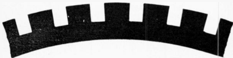
FIG. 1,518.—Style of armature core stamping used with bar wound machines. This construction, since there are no indentations in the teeth for wedges, makes it necessary to provide bands to hold the bars in place.
