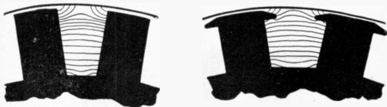
FIGS. 1.427 and 1.428.—Diagram showing respectively the character of stray field between adjacent straight poles, and between adjacent poles with shoes. Across the slightly V-shaped spaces the stray field passes in lines that, save near the outer part, are nearly straight. Quite straight they would not be, even were the sides parallel, because the difference of magnetic pressure increases from the roots towards the pole ends. At the roots, where the cores are attached to the yoke, the magnetic pressure difference is almost zero. It would be exactly zero if there were not a perceptible reluctance offered by the joints and by the metal of the yoke. The reluctance of the joint causes a few of the lines to take paths through the air by a leakage which adds to the useful flux. At the tops of the cores there is a difference of magnetic pressure equal to the sum of the ampere-turns on the two cores, tending to drive magnetic lines across. This difference of magnetic pressure increases regularly all the way up the cores from root to top; hence, the average value may be taken as equal to the ampere turns on one core. The stray field, therefore, will steadily increase in density from the bottom upwards. In addition to this stray field between the pole cores there is also a stray field between the projecting tips or edges of the pole shoes, as shown in fig. 1.428. In some machines the dispersion due to the pole shoes is greater than that between the flanks of the cores.
