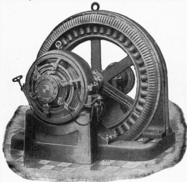
FIG. 1433.—Fort Wayne alternator with direct connected exciter mounted on the field shaft at such distance as to permit a pedestal and bearing to be mounted between the exciter and revolving field. In the view, the bearing is hidden by the exciter, only the foot of the pedestal being visible.
