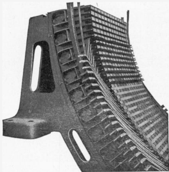
FIG. 1,484.—Section of General Electric stationary armature showing method of assembling the coils. These are form wound and are held in the slots by suitable wedges, the open slot construction permitting the use of form wound coils that can be easily removed and replaced in case of damage. Where heavy windings project beyond the laminations, an additional support is provided by means of an insulated metal ring, to which the outer ends of the coils are fastened; the coils are thereby protected from mechanical displacement, or distortion due to the magnetic disturbances caused by violent fluctuations of the load or short circuits. The figure shows a section of a supporting ring of this type and indicates the method of connecting the coils to it. In order to admit of the prompt replacement of damaged coils, sufficient space is usually provided between the alternator bearings to allow ample movement of the armature to permit of ready access to both armature and field coils. Where space necessitates the use of a short shaft, access to the windings may be had by disconnecting some of the coils and lifting the upper half of the armature.
