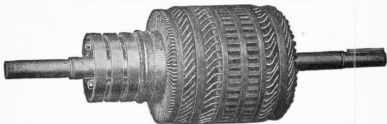
FIG. 1,453.—Port Wayne armature for self-excited alternator. There are two independent windings, one for the main current, and one for the exciting current. The winding for the latter current occupies a very small amount of space, and is placed in the slots on top of the main winding. The commutator to which the exciter winding is connected, is located between the collector rings and the core. It is of standard construction with end clamps holding the bars in place on the insulated commutator drum. The armature coils are form wound and the core is built of sheet steel laminations, annealed and japanned to prevent hysteresis and eddy current losses. Ventilated openings are provided to allow a free circulation of air both around the ends of the windings and through ducts in the laminated core. The core is clamped by bolts between the flanges of the armature spider which is keyed to the shaft. These flanges have cylindrical extensions with ribbed surfaces, which form a support for the ends of the armature coils. The ribbed surfaces form air passages from the core outward around the ends of the coils, thus ventilating both core and coils.
