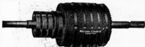
FIG. 1,430.—Western Electric armature for self-excited alternator. The main winding is placed at the bottom of the slots, each coil being surrounded by an armour of horn fibre. The exciter winding occupies a very small portion of the slot, being placed on top of the main winding, and connected to the commutator immediately in front of the core and between core and collector rings as shown.
