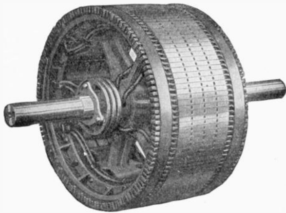
FIG. 1,800.—Allis-Chalmers phase wound external resistance type or slip ring armature construction. The winding is for three phases and the terminals are brought out to three slip rings. The front bracket is slightly modified to make room for these rings on the inside. For starting duty sufficient resistance is supplied to reduce the starting current taken by the motor to 1\frac{1}{2} times the normal full load current. In the running position the resistance is all cut out of the circuit. For speed regulation sufficient resistance is supplied to reduce the speed 50% on normal full load torque.
