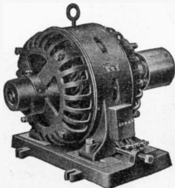
FIG. 1,650. —Ideal fifteen horse power two phase induction motor. The armature core is supported by a cast iron frame carried on a base, with sliding ways and screw adjustment for tightening the belt. The armature core is provided with ventilating apertures, with metal spacers between each tooth. The revolving field is a steel casting with radially projecting poles, to which the pole shoes are bolted. The overhanging pole tips retain the field coils. All coils of the smaller sizes are wound with insulated copper wire of square section, and of the larger sizes, with flat copper, wound on edge, each turn being insulated by sheet insulation. Motors of this type are adapted for use in small power plants and isolated plants. The relatively high speed for which they are designed, reduces considerably the weight and overall dimensions, and likewise the cost. The exciter is belt driven. The normal kw. capacity of the exciter usually exceeds the kw. required for the excitation under normal load conditions to permit of station lighting. All exciters are built as compound wound dynamos, capable of delivering the exciter current up to 125 volts, which is sufficient margin in the field to control the alternating current line voltage on circuits of unusually low power factor.
