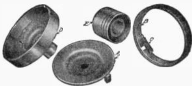
FIGS. 1,852 to 1,855.—Parts of General Electric centrifugal clutch pulley as used on clutch type, single phase induction motor. A, clutch; B, friction band; C, adjusting spring; D, outer clutch shell with pulley sleeve; E, solid removable pulley; F, internal mechanism comprising parts A, B, and C; G, outer shell and pulley comprising parts D and E.
