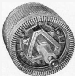
FIG. 1,764.—Western Electric wound armature for internal resistance induction motor. In starting the inductors are short circuited through a resistance which is gradually cut out as the motor comes up to speed.
