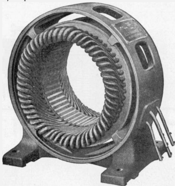
FIG. 1,652.—Armature of Allis-Chalmers squirrel cage induction motor. The frame casting is of the box type and has large cored openings for ventilation. Lugs are cast on the interior surface of the frame to support the core, leaving a large air space between.
