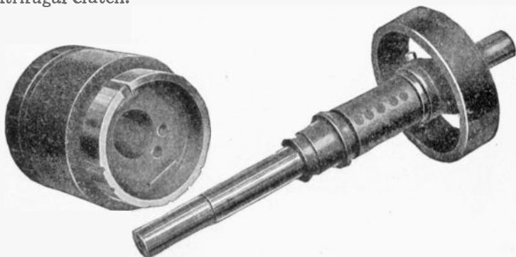
Figs. 1,867 and 1,868. —General Electric dissembled clutch as used on clutch type, single phase (KS) induction motor. In starting, the armature revolves freely on the shaft until approximately 75 per cent. of normal rated speed is reached. The load is then picked up by the automatic action of a centrifugal clutch, which rigidly engages an outer shell, keyed directly to the shaft. The brass friction band of the clutch is permanently keyed to the pulley end of the armature.
