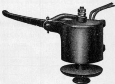
FIG. 2,272.—General Electric low voltage attachment for circuit breakers. This low voltage trip is designed to operate the circuit breaker when the line voltage drops to approximately 50 per cent or less of the normal voltage. It should be noted that the coil is always in circuit, as is the case with the overload and underload coils, and that it operates with the releasing of its armature. It is always necessary to use a fixed amount of resistance (depending upon the voltage of the system) in series with the low voltage release. The low voltage release performs the functions of a shunt trip coil when used in conjunction with a push button, auxiliary switch or speed limiting device, and is generally preferred to the shunt trip attachment.
