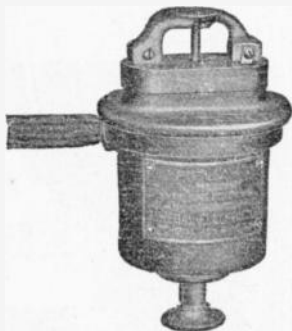
FIG. 2,301.—Alternating current low voltage circuit closing low voltage relay, for 600 volts or less. The contacts are similar to those of the circuit closing overload type except that they are inverted. As long as the pressure is normal the contact cone is held above the contacts. When the pressure falls below one half normal, the cone and plunger rod drop and close the contact. This relay does not pick up its own plunger. The plunger rod is pushed up by hand after the pressure circuit is established. Low voltage relays are generally used in connection with a low voltage release or shunt trip coil on an oil switch or a circuit breaker. They are used in connection with motor booster sets to prevent a disastrous speed of the booster which might result from the loss of alternating current power. They are also sometimes used for indicating purposes.
