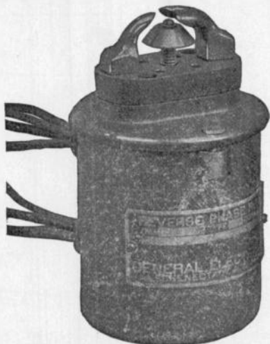
FIG. 2,306.—Alternating current series reverse phase single pole, circuit closing, two contact relay for 600 volts or less. This type of relay is used chiefly to open motor circuits for elevators to prevent damage in case of reversal of leads in reconnecting wiring to two or three phase motors. The relay is provided with a dust proof metal cover.
