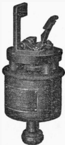
FIG. 2,305.—General Electric direct current solenoid control relay. Solenoids for operating large switches, etc., frequently require comparatively large operating currents in the "closing" coils. This necessitates the use of relatively heavy leads between the control switch and the solenoid and is the cause of severe arcing at the control switch, especially with solenoids of high inductance. These objectionable features can best be eliminated by the use of a suitable control relay located near the solenoids. The control relay consists of a solenoid plunger and switch, the latter insulated from the frame of the relay. It operates satisfactorily on one-half the rated voltage and requires only a very small operating current. The terminals of the switch and the relay coils are independent. The relay can be wound for operation on 125, 250, or 600 volt circuits.
