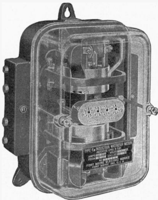
FIG. 2,537. —Fort Wayne multiphase induction watt hour meter. The construction of the mechanism is essentially two single phase motor elements, one at the bottom of the meter in a suitable position, the other inverted and placed at the top of the meter. Each element acts on a separate cup, but both cups are mounted on a single shaft so that the registration is due to the resultant torque of the two elements. The meter is provided with three supporting lugs, the one at the top being keyholed and one of the bottom two, slotted to facilitate leveling. The registering mechanism is mounted on a cast iron bracket at the middle of the meter between the two motor elements. The supporting bracket is attached to the meter base by two screws and aligned by two dowel pins. The register is of the four dial type, reading in kilowatt hours. Each division of the right hand circle, or that passed over by the most rapidly moving pointer, equals one kilowatt hour in meters without a dial constant. In meters of larger capacities, dial constants of 10, 100 and 1,000 are used, in which case it is only necessary to add one, two or three ciphers to the observed reading.
