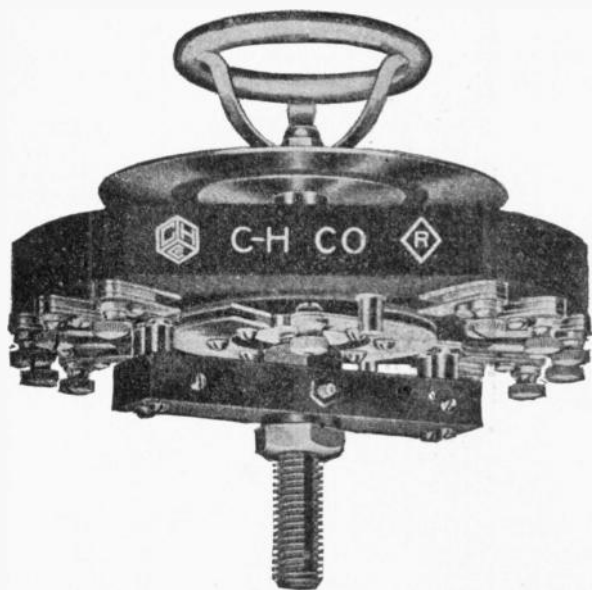
FIG. 2,660.—Crouse-Hinds radial ammeter switch, arranged for mounting directly on the switchboard. It is designed for use with external shunt ammeters of any make or capacity, and in connection with the required number of shunts, makes possible the taking of current readings of a corresponding number of circuits by means of one ammeter. The wiring diagram is shown in fig. 2,670.
