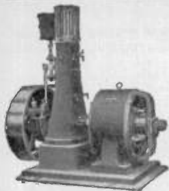
FIG. 2,769.—Triumph direct current generator set with upright slide valve engine.
