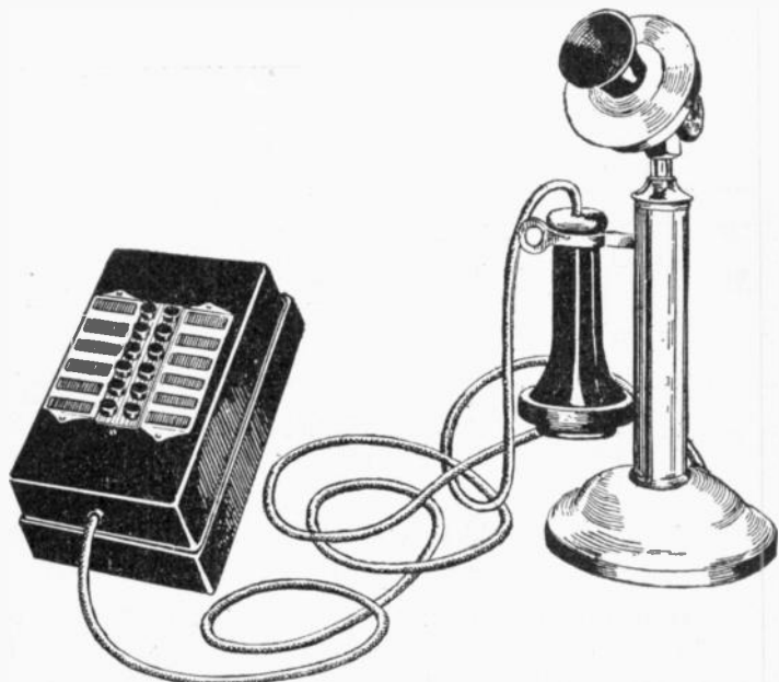
FIG. 2,973. —Western Electric automatic intercommunicating telephone set. This type of instrument is for general use where a high grade of intercommunication is desired. There can be as many stations in the system as there are connected station buttons on the inter-telephone box connecting set. Four additional buttons are connected with the others where the system is used for intercommunicating residence service and connected to a telephone central line. One of these is marked "ring," another "answer," another "transfer," and another "central," depressing any one except "ring" cuts out and automatically restores any other that may be depressed. The "ring" button does not stay depressed like the others. The system permits of any station calling any other and is non-interfering. Several conversations may be carried on at one time between several stations.
