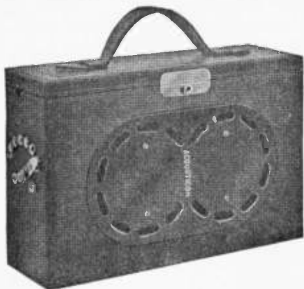
FIG. 3,048.—Type R F acousticon suitable for those who lose most of the words in conversing with one person, even when the voice of the speaker be raised. This type cannot be worn upon the clothing. The transmitters are mounted in a black leather covered case, and when closed for carrying, the instrument looks like a kodak.
