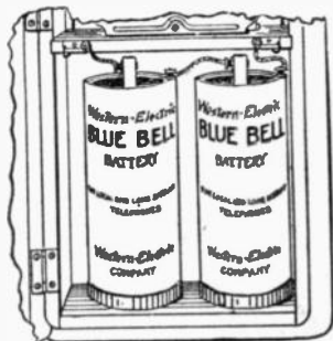
FIG. 2,996.—Installing a magneto set: 3. Connecting the dry cells. For ordinary service two cells suffice, however in the case of long toll connections three cells are recommended. To connect two cells, take one of the loose cords furnished with the set and connect one end to the short outside or zinc terminal, and the other to the long inside or carbon terminal. Place the cells in the lower part of the set and connect the ends of the cords hanging from the terminals on the generator shelf, one to the long part of the first cell, and the other to the short part of the cell.
