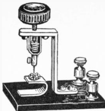
FIG. 3,169.—Crystal detector. When the hard rubber knob at the top of the detector stand is turned, the needle point, which presses into the crystal is moved up or down. This allows of a variable adjustment which may be tight or loose, as desired. The spring shown helps to push the crystal up against the needle point.
