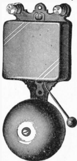
FIG. 3,206.—Bunnell iron box bell. The protection thus secured excludes dust and protects the working parts from injury in exposed places. The armature is pivoted and has adjustable contacts. The resistance of the winding is 4 to 5 ohms.
