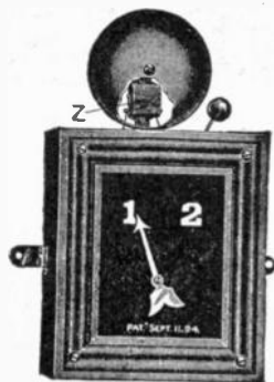
FIG. 3,282.—Automatic annunciator, especially suitable for residence service; it serves the purpose of two bells, one at the front door, and one at the back door. It can be readily converted into a three point annunciator by the addition of the buzzer Z, as shown, which can be operated from the dining room in place of the bell.
