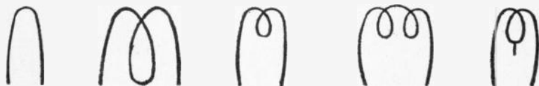
FIGS. 3,481 to 3,485.—Various incandescent lamp filaments. Fig. 3,481 single loop or "U" filament; fig. 3,482, double loop filament; fig. 3,483, single coil filament; fig. 3,484, double coil filament; fig. 3,485, oval single coil anchored filament. The distribution of light from an incandescent lamp depends almost entirely upon the shape of the filament. Single loop or "U" filaments emit only about 5 candle power in the direction of the tip, while the single coil filament, having the same mean horizontal candle power emits about 6.6 candle power from the tip. Since incandescent lamps are usually placed with the tip downward it is evident that the amount of light emitted from the tip constitutes what may be called the "useful light," and it is, therefore, of greater importance than the amount of light emitted in any other direction. It is obvious that the "U" shaped filament emits less light in the direction of the tip than the coil filament for the reason that it exposes less surface in that direction than the latter, therefore, in order to increase the candle power in the direction of the tip, it appears necessary only to increase the number of coil of the filament. It will be noted in this connection, that in the case of the double coil filament, the distribution of light in the vertical plane is 8 candle power from the tip. It must be clearly understood, however, that in practical illumination, incandescent lamps are arranged not only with their tips pointing vertically downwards, but also in many other directions, and that in such cases various kinds of reflector, globe and shade are employed to throw all the light emitted by the lamp in a given direction, or to aid in giving a uniform distribution.
