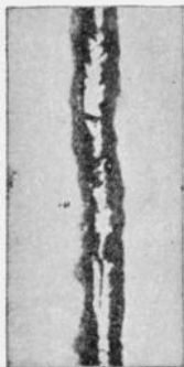
FIGS. 3,438 to 3,440.—Behavior of tantalum filament. Fig. 3,438, unburned tantalum filament; fig. 3,439 tantalum filament after burning 800 hours on direct current; fig. 3,440, tantalum filament after burning 800 hours on alternating current. The new filament is smooth and without regular structure, while after burning for some time, it begins to take on a crystalline appearance. This change takes place less rapidly with direct than with alternating current, so that the life of the lamp is somewhat greater in the former case. When the filament finally burns out, it is supposed to be due to the change from the amorphous to the crystalline state, as indicated in the illustrations.
