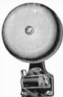
FIG. 3,204.—Mesco single stroke bell. The hammer rod has a short leverage but a long sweep, thus enabling it to give rapid and powerful blows. A stiff flat spring causes the hammer to leave the bell immediately after striking. The magnets of this bell are regularly wound for 6 ohms, and special for incandescent lighting circuit. Sizes 3 to 18 inch.
