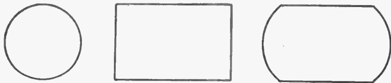
FIGS. 3,882 to 3,884.—Various film perforations. These are called: fig. 3,882, round; fig. 3,883, square; fig. 3,884, barrel. The square and barrel holes seem to be more durable than the round hole. The shape of the holes should correspond to the shape of the sprocket teeth. A standard perforation is four pairs of holes per picture, each hole being approximately \frac{1}{16} \times \frac{1}{16} , spaced along the edges of the film \frac{1}{16} inch apart, making four holes at each edge for a \frac{1}{4} inch motion picture image.
