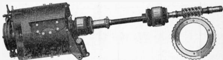
FIG. 4,082.—Baker R and L motor, propeller shaft, universal joints, worm and gear. This is the straight type top mounted worm drive.
