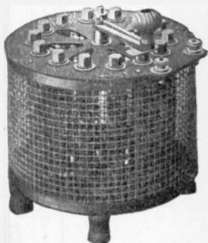
FIGS. 3,879 and 3,880.—Powers' rheostats. The type shown in fig. 3,879 is designed for use on 110 volt circuits and will carry 25 amperes without overheating. The coils are so supported that any of them may be replaced when desired. Adjustment is effected by means of a lever switch. Fig. 3,880 shows Underwriters' pattern rheostat of 25 amperes capacity. It is designed for 110 volts and is not adjustable.
