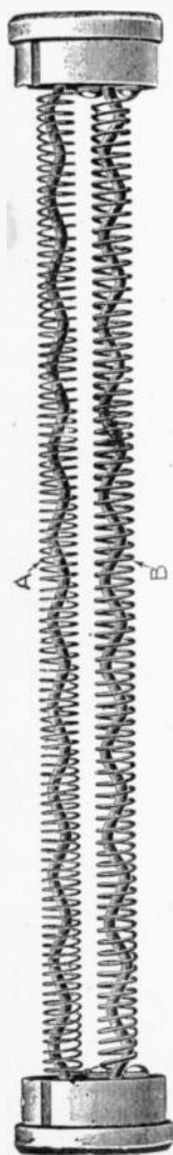
FIG. 3,682.—View showing construction of Gold two coil heater unit. The coils are so designed as to insure a circulation of air. In this heater the coils are wound around wavy metal rods as shown. The smaller coil A provides one-third the heat and the larger coil B, two-thirds, thus making it possible to obtain three variations in the amount of heat furnished, to meet changes in air temperature conditions.
