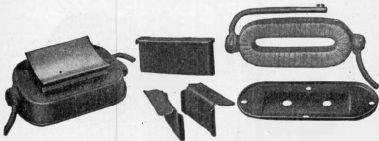
FIGS. 3,542 to 3,547.—Various construction details of General Electric commutating pole railway motor, fig. 3,542, exciting field coil and supports; figs. 3,543 to 3,545 details of commutating field coil and supports; fig. 3,546, brush holders; fig. 3,547, malleable iron gear case.
