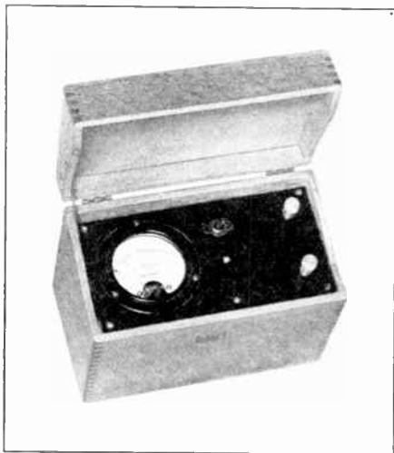
Fig. 2—V. T. Voltmeter Mounted in Card-File Case
