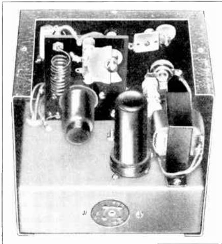
FIG. 51. Interior View, Showing Coil and Condenser Support, Also Horizontal Mounting of 6C5.
