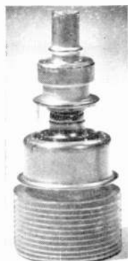
A 2C39A disc seal transmitting valve. (Photo by courtesy of S.T. & C. Ltd).
