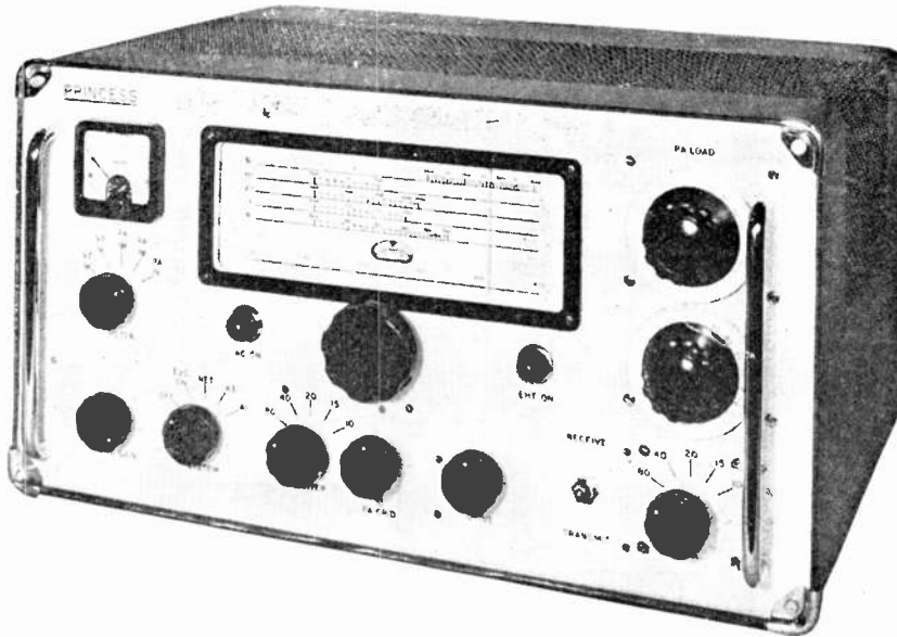
The Princess transmitter employing a mixer master oscillator and linear p.a. stage for c.w. and a.m. operation.
