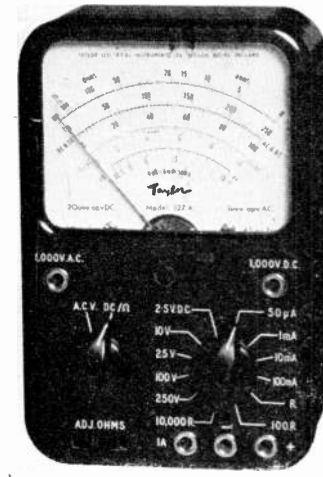
The Taylor Model 127A multimeter with a sensitivity of 20,000ohms per volt. The instrument has 20 ranges and measures resistance up to 20 Megohms. (Photo by courtesy of Taylor Electrical Instruments Ltd.)
