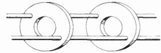
Fig. 14.3. Open-wire line with disc insulators. The centre portions of the insulators are removed to minimize dielectric losses.
