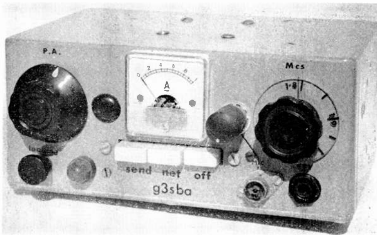
Transistor transmitter for 1·8-2 Mc/s.
