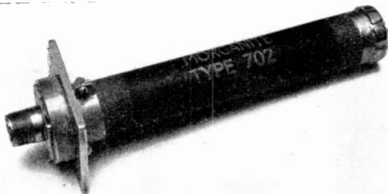
A 25-watt dummy load for 145 Mc/s.
