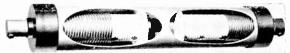
A suitable trap design for multiband rod aerials. (By courtesy of Mosley Electronics Ltd.)
