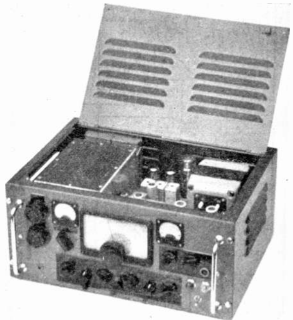
The TT21 transmitter for the 14, 21 and 28 Mc/s bands.
