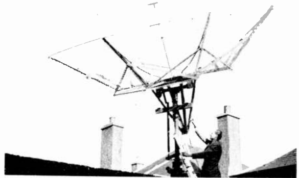
Example of an amateur built parabolic aerial.
