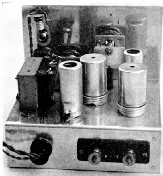
A rear view of the t.r.f. receiver. The components may be identified by reference to Fig. 4.74 (b).
