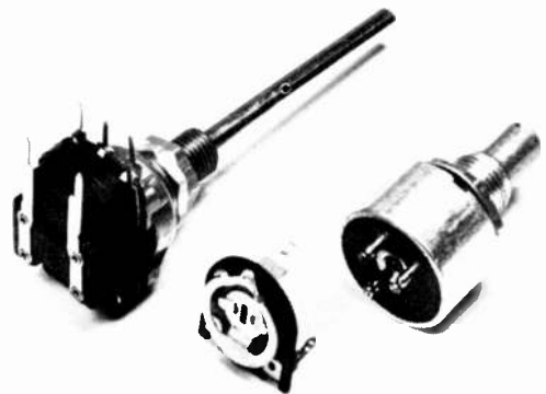
Potentiometers (variable resistors). Left to right: the type commonly used as a volume control with an on-off switch built-in, skeleton preset for pcb mounting, screened preset for chassis mounting.
