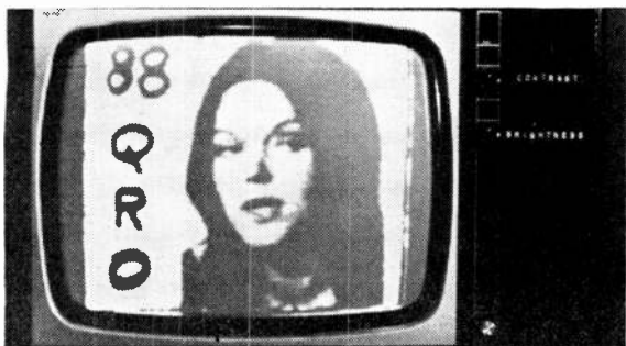
SSTV picture received on a domestic tv set after slow-scan to fast-scan conversion.
