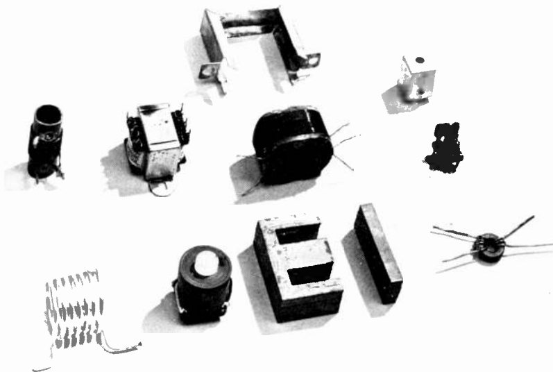
Various inductors. Top left: rf coil on paxolin former and loud-speaker transformer. Bottom left: self-supporting silver-plated vhf coil and Ferroxcube-potted high-Q coil. Centre: exploded view of mains transformer, showing two-part laminated iron core, coil former and aluminium cover. Top right: i.f. transformer with and without its screening can. Bottom right: small toroid transformer for use at rf.
