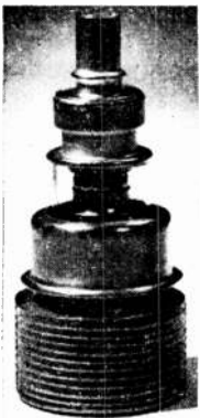
A 2C39A disc seal transmitting valve. (Photo by courtesy of S.T. & C. Ltd).
