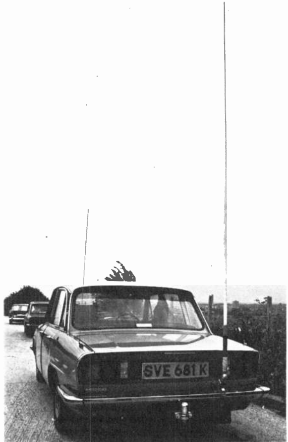
Two-aerial installation. Left: 70MHz \lambda/4 whip; right: 7MHz helical whip with a base-loading coil for 1.8MHz.
