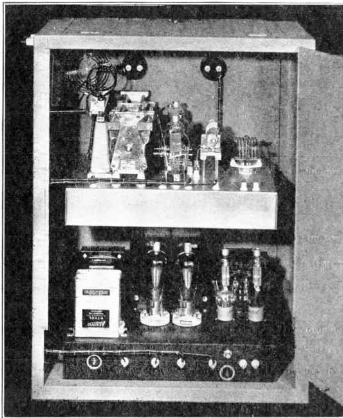
Figure 14. REAR VIEW OF R.F. AMPLIFIER AND MODULATOR.
