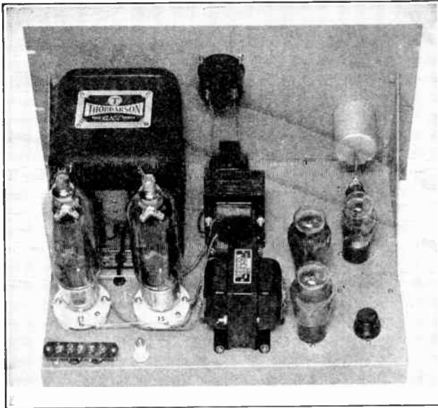
Figure 18. 203-Z SPEECH-MODULATOR FOR INPUTS TO 800 WATTS. The complete speech amplifier and class B output stage are built upon a single relay-rack panel and its associated chassis. The speech amplifier incorporates automatic peak limiting and uses a pair of 2A3's as drivers for the 203-Z's.
