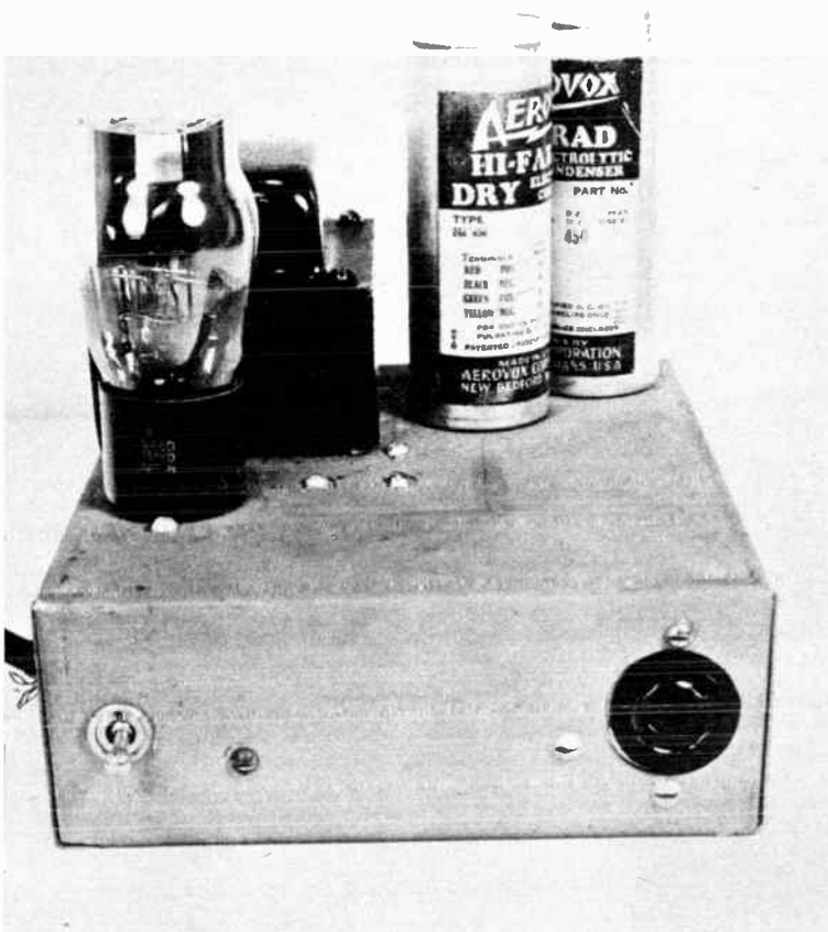
Figure 19. SHOWING METHOD OF CONSTRUCTION OF A SIMPLE LOW-VOLTAGE RECEIVER OR FREQ.-METER POWER SUPPLY. The circuit diagram of this unit is given in Figure 20.
