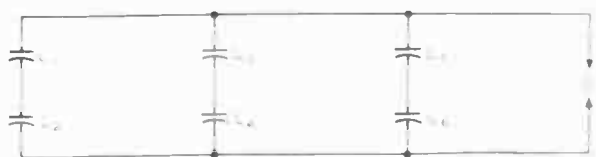
CAPACITORS IN SERIES-PARALLEL
