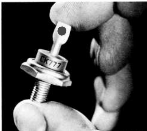
Figure 14 MINIATURE SEMI-CONDUCTOR TYPE RECTIFIER
