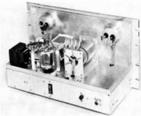
Figure 24 REAR OBLIQUE VIEW OF PI-COUPLED AMPLIFIER
