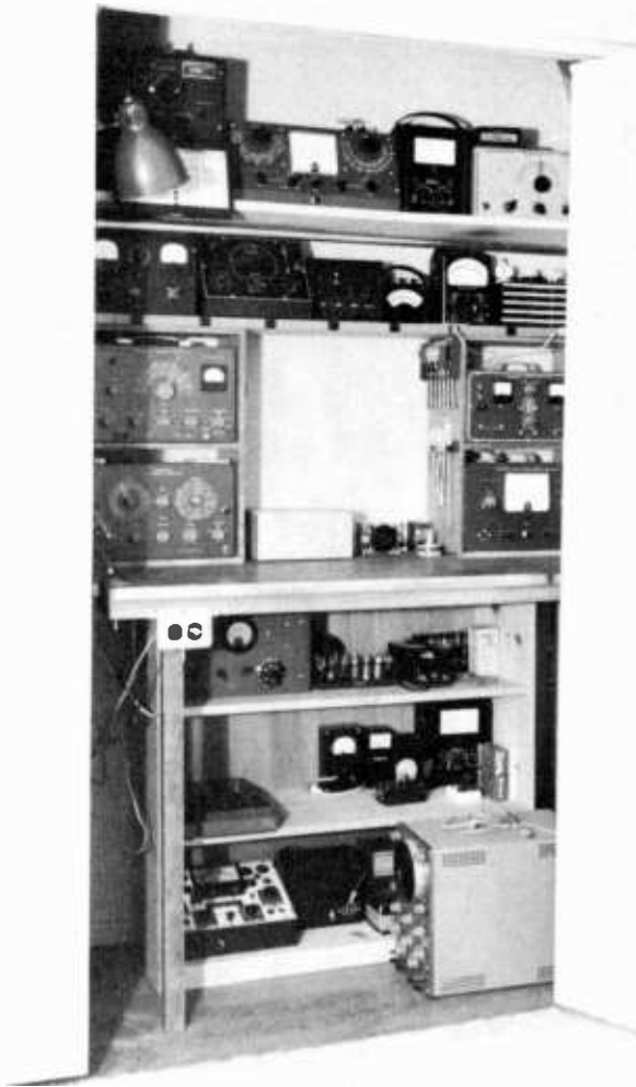
Figure 13 COMPLETE WORKSHOP IN A CLOSET! Careful layout permits complete electronic workshop to be placed in one-half of a wardrobe closet. Work bench is built atop an unpainted three-shelf bookcase.
