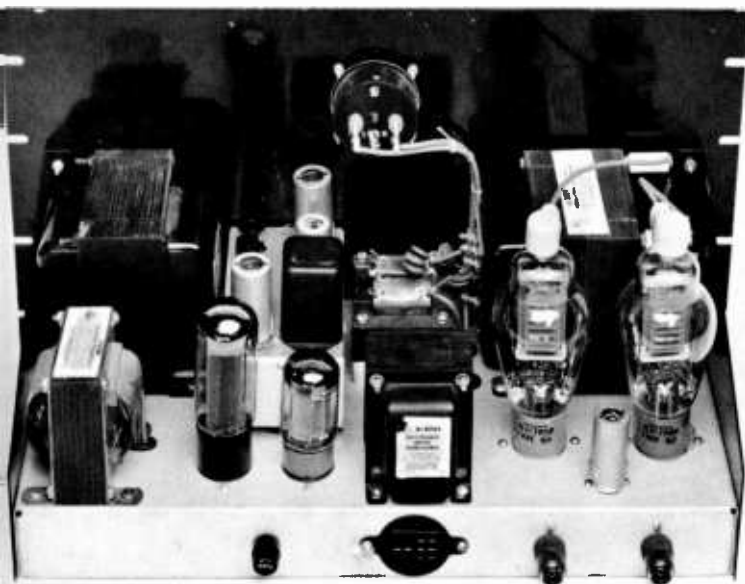
Figure 16 REAR VIEW OF 811-A MODULATOR Modulator tubes and voltage regulator are at right with high level filter at center of chassis. Plug-in speech amplifier is to left of clipper. Gain and clipping controls are atop the small chassis. 6L6/5881 is used as cathode follower driver stage for modulator.
