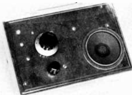
Figure 4 TWO TRANSISTOR BROADCAST RECEIVER IS EXCELLENT BEGINNER'S PROJECT
