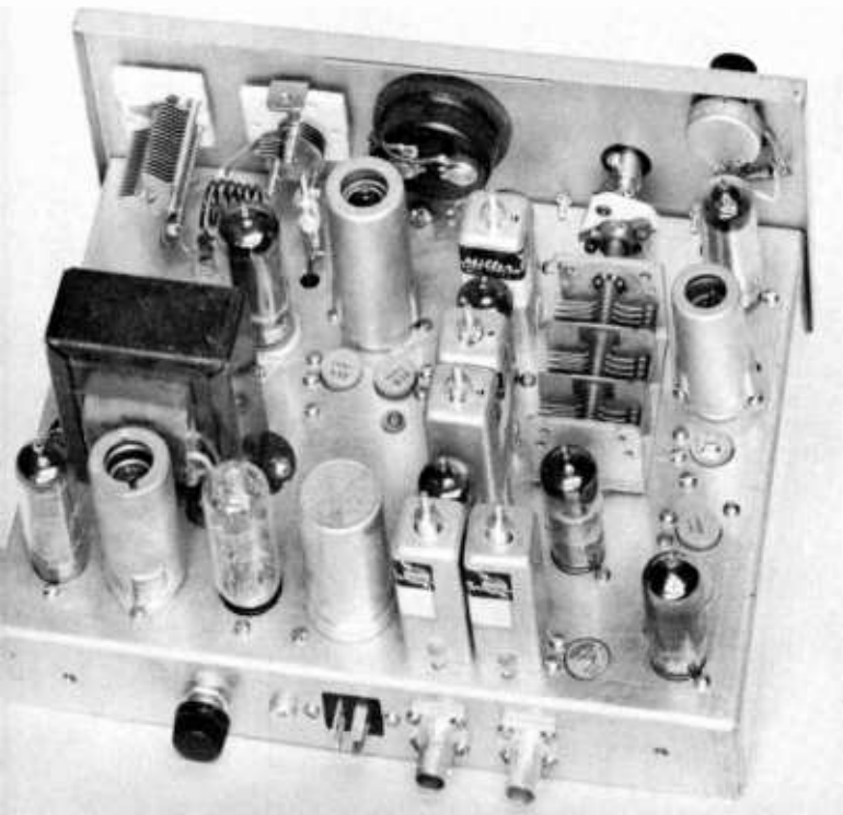
Figure 33 REAR VIEW OF SIX METER TRANSCIVER CHASSIS
