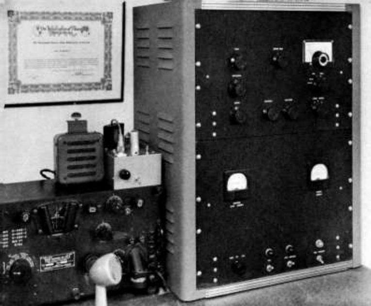
Figure 1 COMPACT 300 WATT TRANSMITTER FOR SIX AND TWO METERS IS IDEAL FOR VHF ENTHUSIAST
