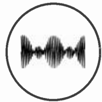
Figure 6 THREE-TONE SSB ENVELOPE WHEN EQUAL TONES OF EQUAL FREQUENCY SPACINGS ARE USED.
