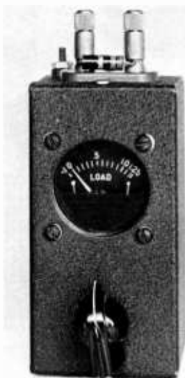
Figure 25 SIMPLE SILICON CRYSTAL NOISE GENERATOR
