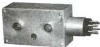
Acorn Tube R-F Plug-In Unit for Perrine Super.
