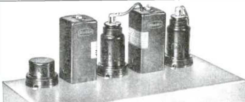
Compact I-F Amplifier with metal tubes and Aladdin midget iron-core I-F transformers.
