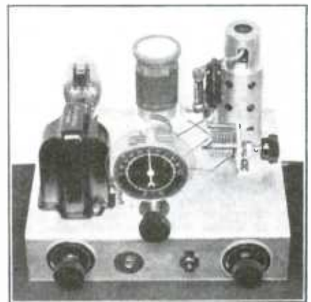
The AC "Gainer" with front panel removed to show correct arrangement of parts.
