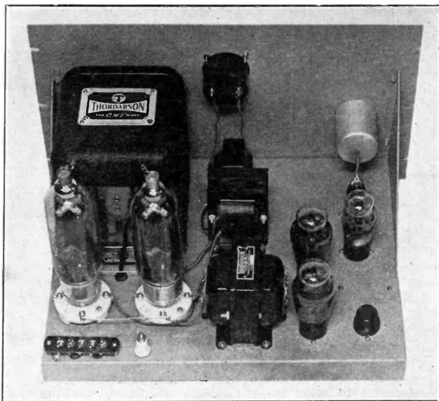
Figure 19. The speech amplifier and 300-watt modulator are contained in one rack unit. The shield on the back of the panel encloses the input jack, bias cell, grid resistor, etc.
