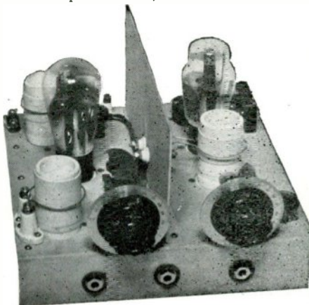
Crystal oscillator link coupled to buffer or doubler stage. 12 gauge aluminum is used. A single aluminum shield is shown between the two stages. Better practice dictates the use of a double shield, with \frac{1}{4} -inch spacing between shields.
