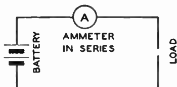
AMMETER CONNECTED IN CIRCUIT
