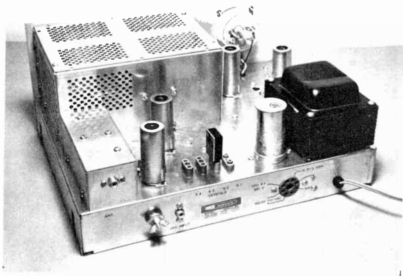
11-4. Back view of completed DX-60B transmitter with cover of cage in place. One crystal is in position, at jack X 2 .
