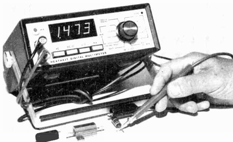
15-12. Completely solid-state, this digital-type test meter features direct readout on all its measurement functions.
