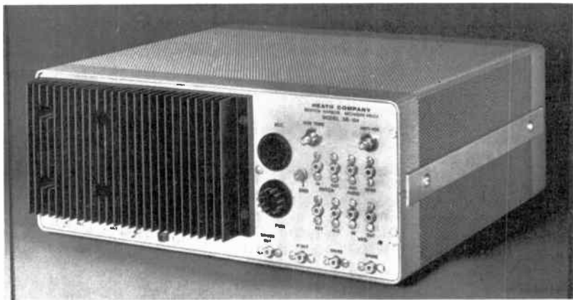
11-12. Back view of the transceiver. The dark area at the left is a heat radiator for the power transistors of the transmitter section.
