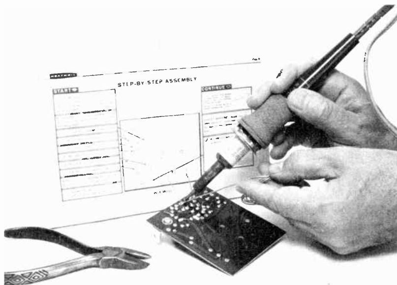
10-3. Transistors, resistors and capacitors of the oscillator mount through holes in a printed circuit board and are soldered on the bottom side. Iron with a small tip is needed for this work.
