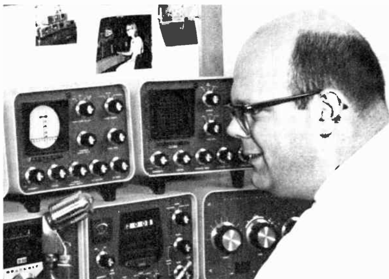
9-15. Two different types of Heath monitor scopes, with 3-inch cathode-ray tubes, enable Alan Robertson, K8BLL, Benton Harbor, Mich., to keep track of received signals and also his own.
