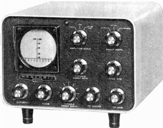
14-13. Small oscilloscope is used to great advantage in this Heathkit Spectrum Monitor to show actual shapes of sent and received signals.
