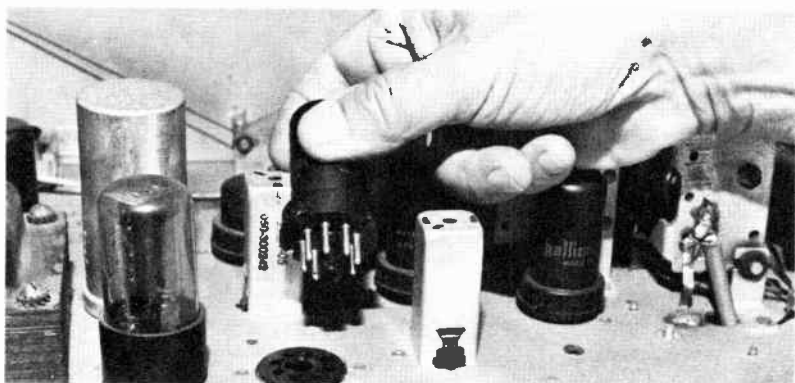
4-15. Then grasp the top of the tube firmly with dry fingers, pull without turning, and it will pop up without damage.
