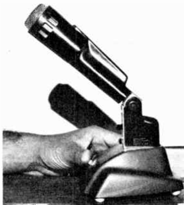
3-16. Typical dynamic microphone (Electro-Voice Model 664) found in amateur stations. Heavy base and rubber feet minimize creeping on table. "Push-to-talk" switch on base actuates control circuits in the transmitter.
