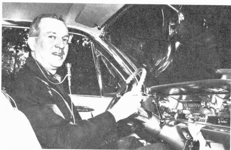
13-4. Bil Harrison, W2AVA, of New York, doesn't take his hands off the wheel when he's out mobiling. He wears a neck mike and has an earplug receiver, and uses his left foot to operate a switch that controls his transceiver. Latter is mounted on floor behind him.
