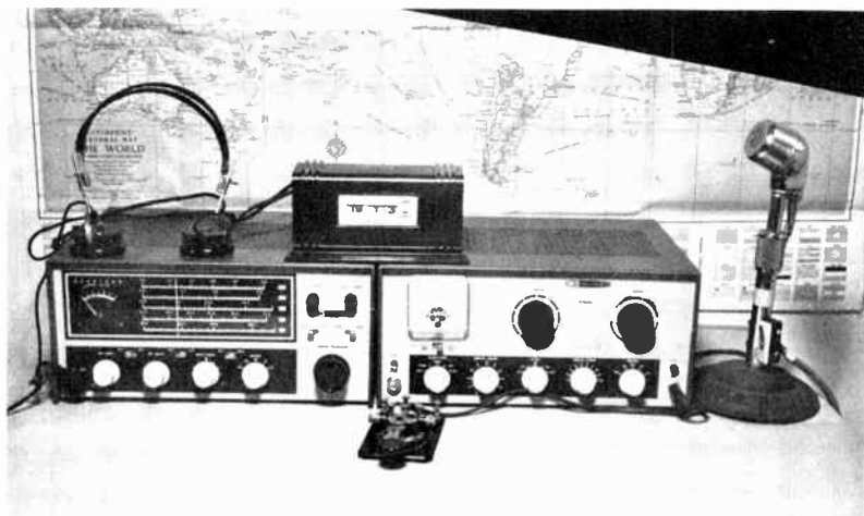
11-6. A complete ham station. HR-10B receiver at left and DX-60B transmitter at right.
