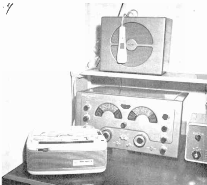
10-4. With this setup of a tape recorder and a shortwave receiver, you can record timed practice transmissions for repeated replaying.
