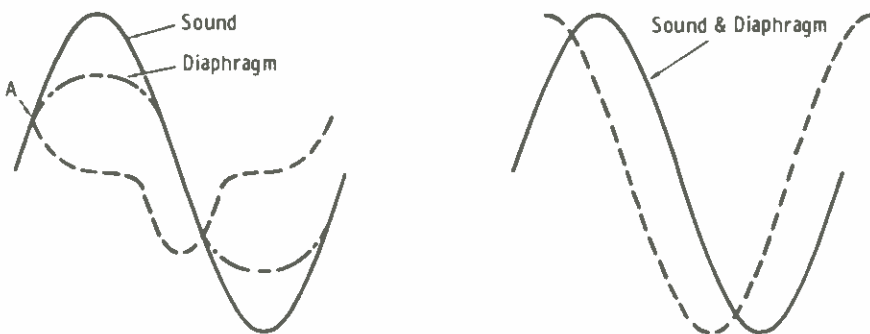
(A) Action under excessive pressure. (B) Action with normal loading.
