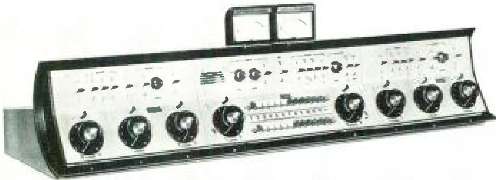
Fig. 6-21. Dual-channel console employing transistor circuitry.
