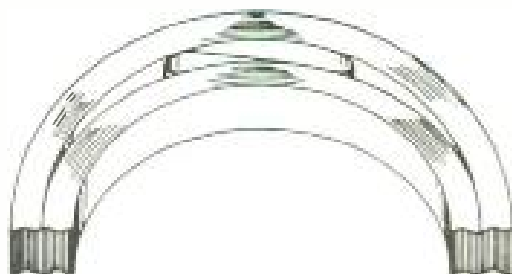
Fig. 13-22. When tape is looped as shown, it must be discarded.
