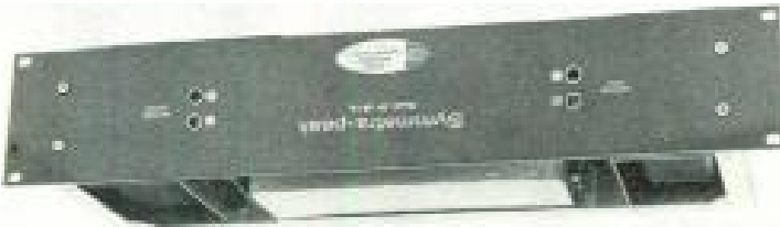
Fig. 14-4. A device for removing asymmetrical energy from audio peaks.
