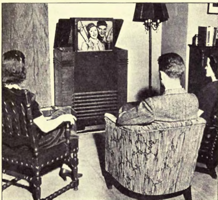
FIG. 55—(Top) a television projection tube. (Below) television picture produced by a projection tube upon a 13x18 inch screen, after magnification by means of a lens system.
