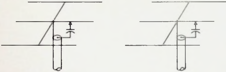
Fig. 3.34 — To keep driven elements in phase with equal length feedlines, gamma matches must be located on same side of antenna element.
