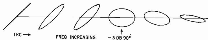
Fig. 431. Input-output comparator response sequence for an amplifier with the stability margin satisfactorily adjusted. (See also Fig. 403.)
