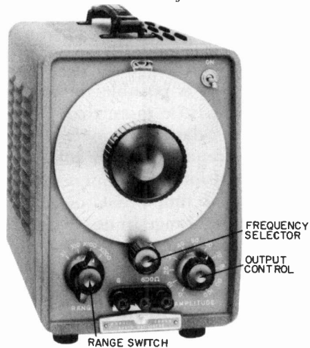
Fig. 206. An R-C oscillator employing the basic circuit of Fig. 204-c. (Courtesy Hewlett-Packard Co.)
