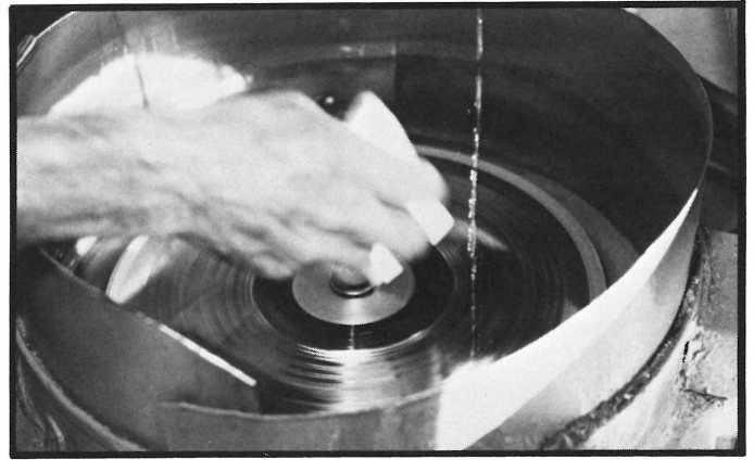
Polishing a metal mother helps get rid of "horns".
