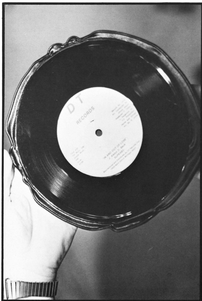
A pressed record before the flash has been trimmed.
