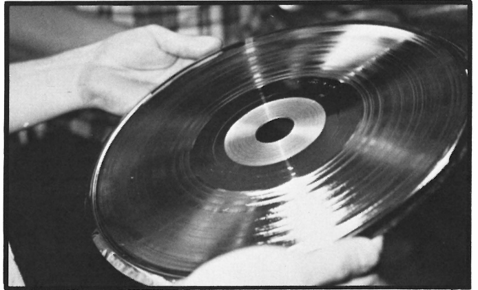
A stamper ready to go to press. Note carefully punched center hole and fluted edge.
