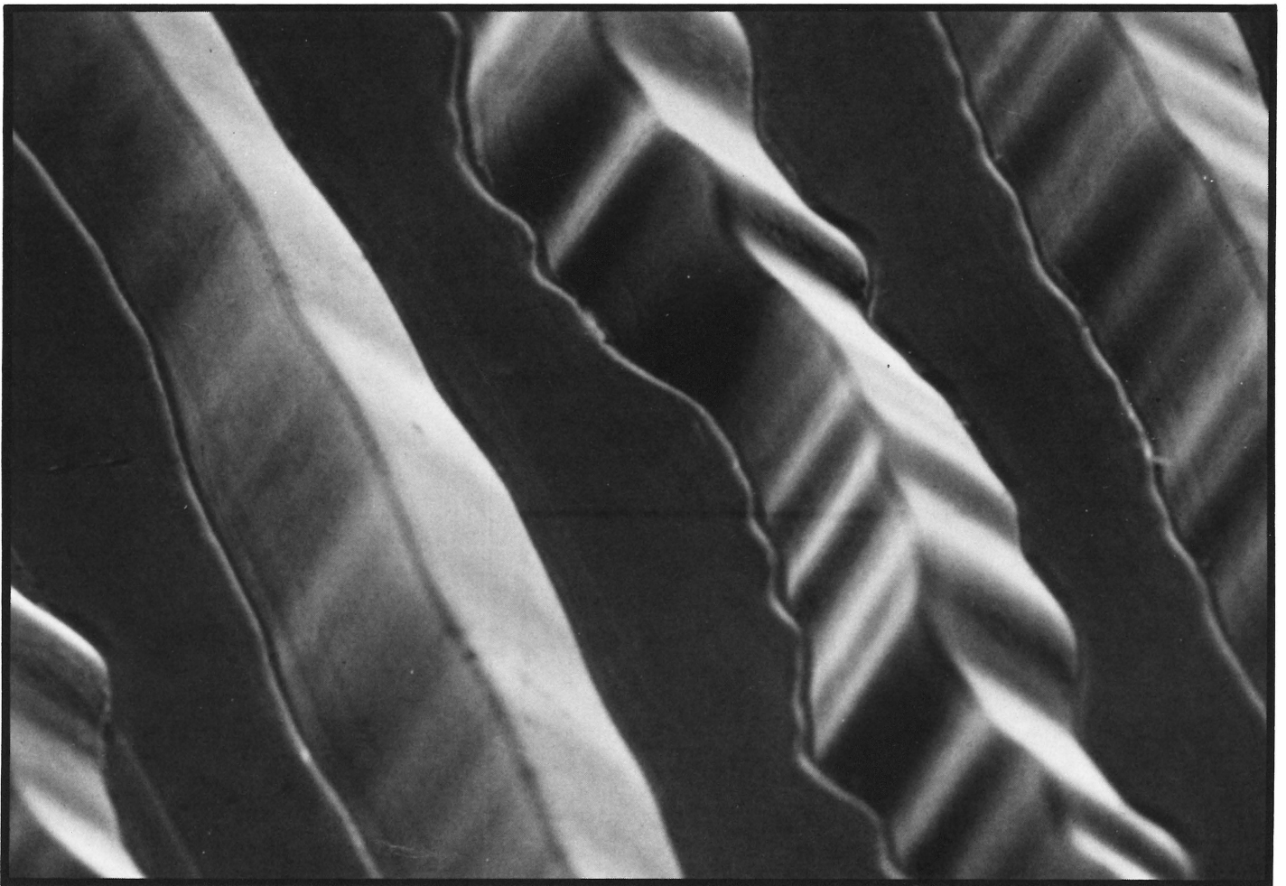
The raised grooves on a nickel stamper. (Photo courtesy Stanton Magnetics)
