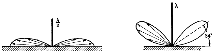
FIG. 8 E. Radiation patterns from vertical Marconi antennas
