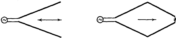
FIG. 35 I. "V" and Rhombic types of antenna
