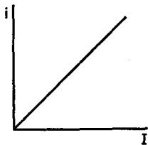
FIG. 20 C. The photoemission i is directly proportional to the intensity of the light, I
