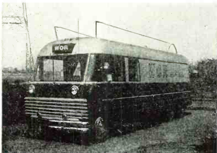
Fig. 10-3. The second link in an on-the-spot broadcast is often a mobile short-wave transmitter installed in a truck.
