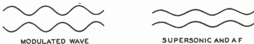
Fig. 4-32. Difference between a modulated waveshape and a combination of the superasonic and audio waveshapes as used in magnetic recording.
