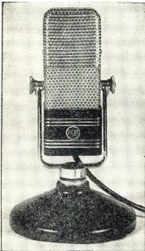
Fig. 18-20. In (A) is shown an external view of a ribbon-type (velocity) microphone. The family of response curves for the ribbon-type microphone is shown in (B). These curves show how the response of the microphone varies for three frequencies at different angles with the microphone.
