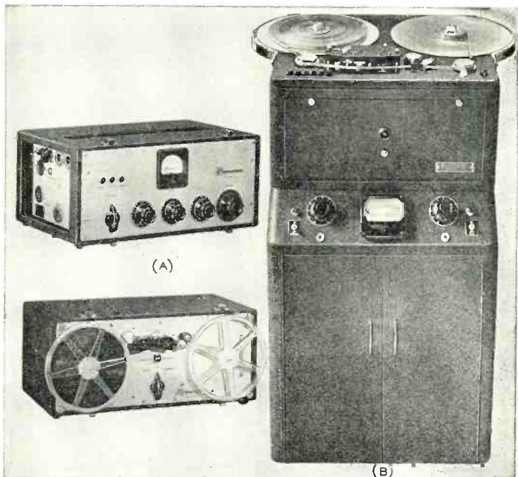
Fig. 4-26. (A), a small portable-type recorder ; (B), a large studio-type recorder.
