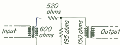
FIG. 24.6. An L-type pad to match a 600-ohm output to a 150-ohm input circuit.
