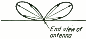
FIG. 20.10. Vertical radiation pattern of a horizontal antenna one half-wavelength above ground. End view of the wire.
