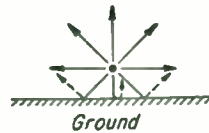
FIG. 20.9. When near the ground, energy is reflected, changing the radiation pattern of the antenna.
