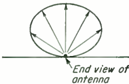
FIG. 20.11. Vertical radiation pattern of a horizontal antenna a quarter-wavelength above ground.
