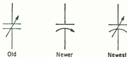
FIG. 6.5. Symbols used to denote variable capacitors.
