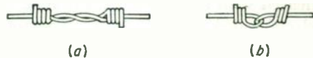
FIG. 1.24. (a) Properly made splice between two ends of wire. (b) Very poor method of splicing two wires.
