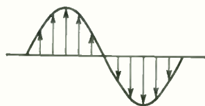
FIG. 4.4. Vectors indicating instantaneous amplitudes every 30^\circ of one cycle.
