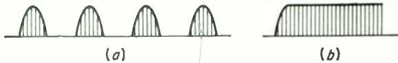
FIG. 10.9. (a) Pulsating d-c is smoothed to (b) pure d-c for use in electronic circuits.
