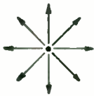
FIG. 20.8. Amplitude of radiation from a horizontal half-wavelength antenna in free space. End view of the wire.
