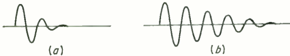
FIG. 12.3. Alternating current damps out (a) rapidly in high-resistance circuits, and (b) slowly in a low-resistance circuit.
