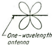
FIG. 20.17. Radiation pattern of a full-wavelength antenna, as seen from above it.
