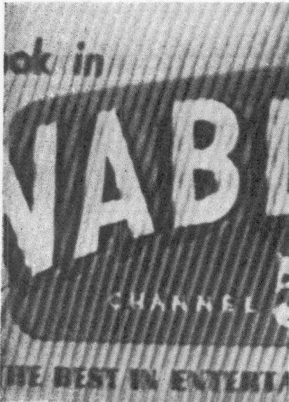
FIG. 1—Interference from third video i-f harmonic on channel 5
