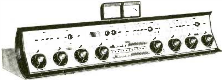
Fig. 6-21. Dual-channel console employing transistor circuitry.
