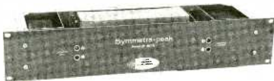
Fig. 14-4. A device for removing asymmetrical energy from audio peaks.
