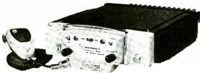
Fig. 13-28. A mobile transmitter-receiver.
