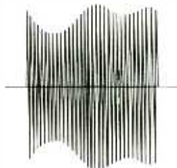
(B) Underbiased single-ended stage.
