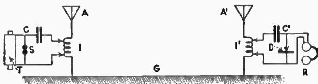
FIG. 1.—Example of a Radio System. A-A', Aerials. C-C', Condensers. T, Transformer Coil. D, Detector. I-I', Inductances. S, Spark Gap. G, Ground. R, Telephone Receiver.
