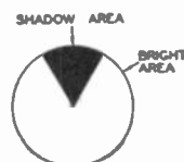
FIG. 6.16C. The eye opening when the grid becomes more positive.
