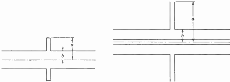
Fig. 9-11e Circular wave guide with shorted radial line in series with cylinder wall.
