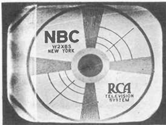
Figure 60—Effect of Damping Tube Failure
