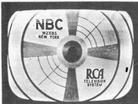
Figure 55—Vertical Distortion Caused By Defective Peaking
