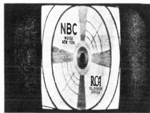
Figure 35—Horizontal Width Control Incorrectly Set
