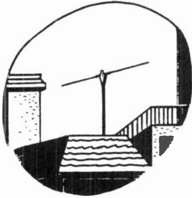
FIG. 47 SINGLE DIPOLE ANTENNA INSTALLATION
