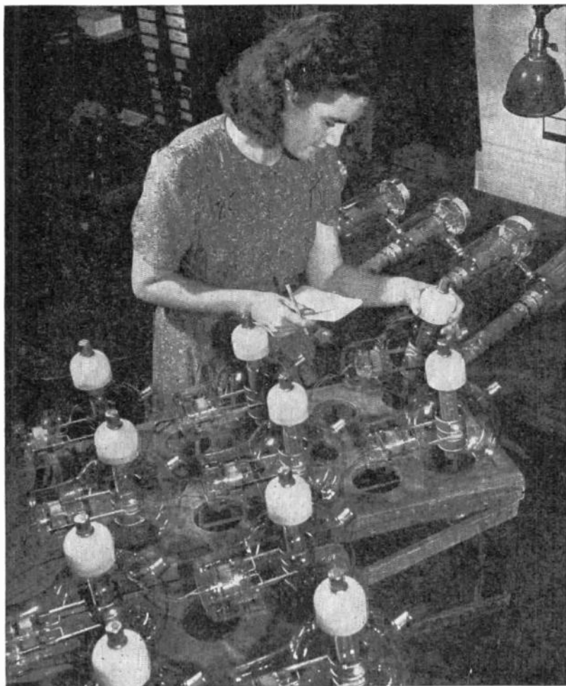
INSPECTING HIGH FREQUENCY RADIO TRANSMITTING TUBES USED IN COMMUNICATING MESSAGES BETWEEN SHIPS AND SHORE RADIO STATIONS. THERE ARE NEARLY THIRTY TYPES OF TRANSMITTING TUBES MADE OF WHICH ONLY TWO ARE SHOWN
