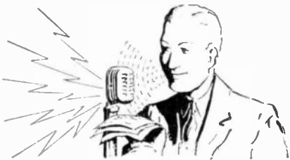
Fig. 1. Diagram Showing Microphone Used to Change Sound Energy into Audio-Frequency Electrical Energy
