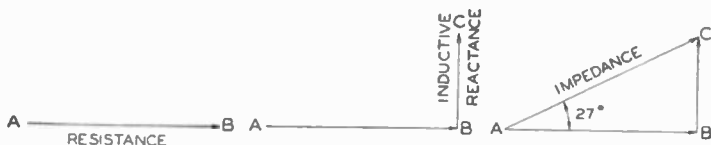
Fig. 4. Diagram Showing the Effect of Resistance and Reactance
