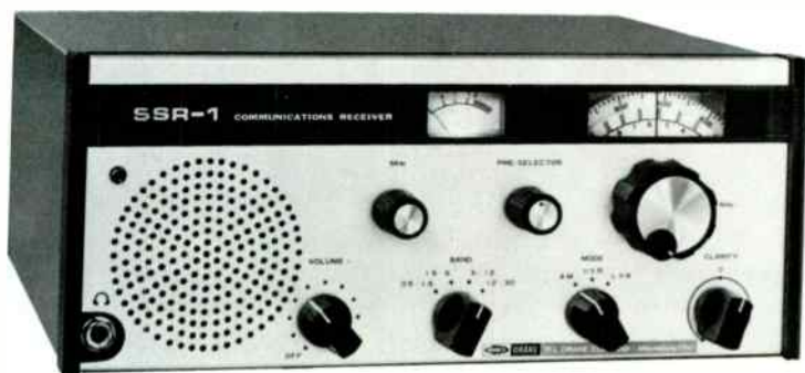
Fig. 4-4 The new Drake SSR-1 is a synthesized, solid-state desk-top 500kHz to 30MHz AM portable. A great new receiver in the $350 class.
